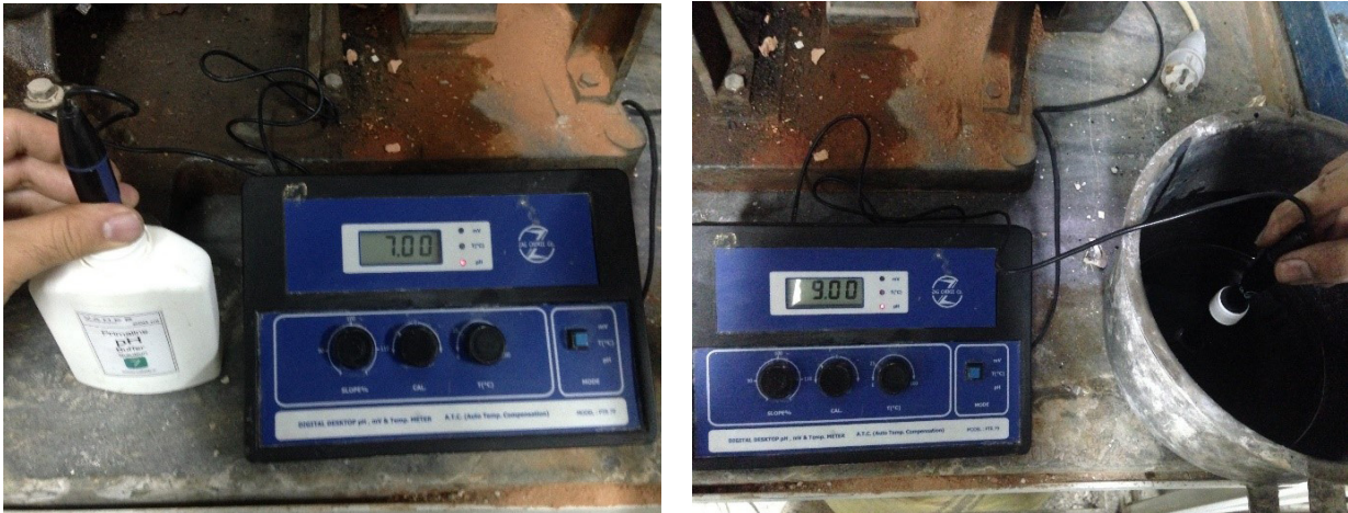
Figure 2. Adjusting pH value of the mixture gel up to 9 for better dispersion of the nanoparticles
