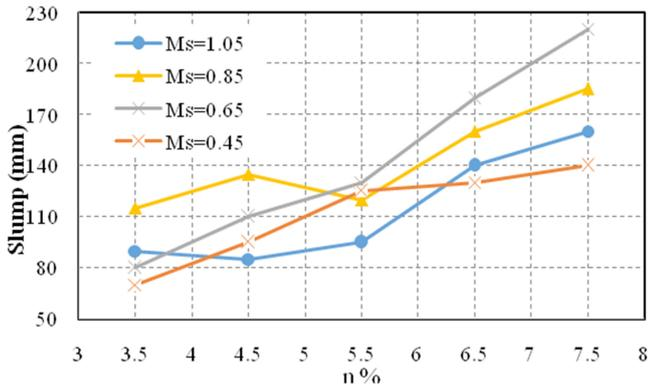
**Fig. 2. The effect of alkali solution parameters on slump of AAS concrete.**
