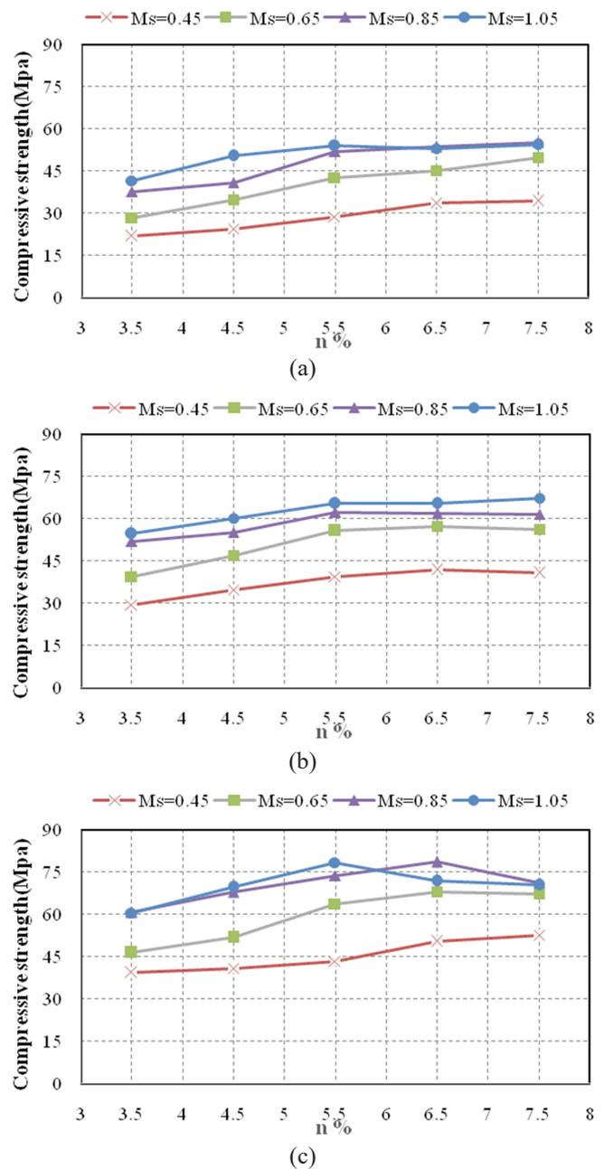
Fig. 1. Compressive strength of AAS concrete based on activator modulus and activator concentration: (a) 7- day; (b) 28-day and (c) 90-day compressive strength.
