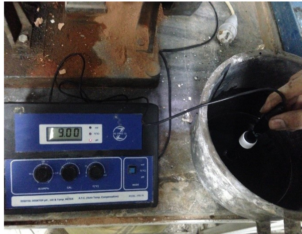
Figure 2. Adjusting pH value of the mixture gel up to 9 for better dispersion of the nanoparticles
