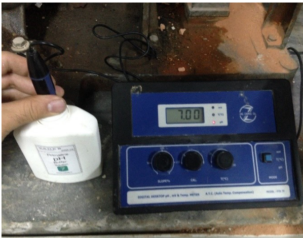
Figure 2. Adjusting pH value of the mixture gel up to 9 for better dispersion of the nanoparticles
