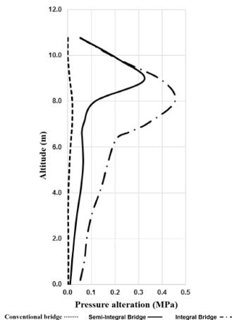
**Figure 7. Soil pressure-drop pattern in abutments with active soil**
