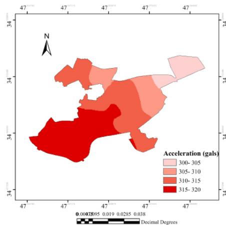
Figure 8. Micro-zonation of average horizontal  $S_a$  at 0.1 sec. and bedrock with earthquake return period of 975 years
