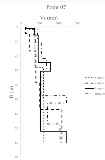
**Figure 15. Shear wave velocity profile for the point 7 from four initial model with 3, 5, 7, and 10 layers by inversion of H/V spectrum**
