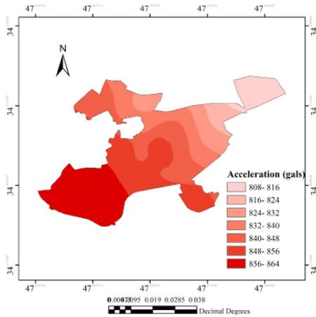
Figure 10. Micro-zonation of horizontal PGA at bedrock with earthquake return period of 475 years
