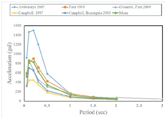
Figure 5. Uniform hazard spectra for center of Kangavar at bedrock with earthquake return period of 975 years
