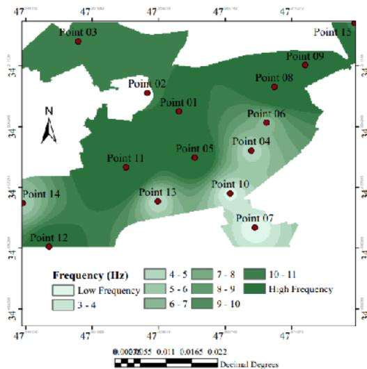
Figure 13. Micro-zonation map for natural frequency of the ground with location of ambient vibration measurements
