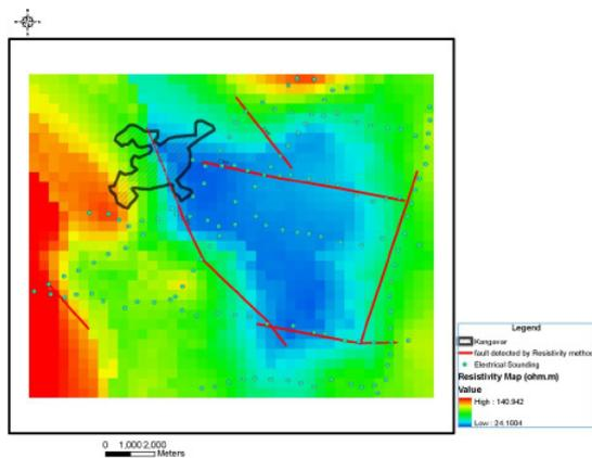
Figure 17. Semi-electrical resistivity map of Kangavar with locations of the sounding profiles
