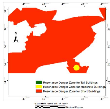
Figure 18. Construction guideline based on amplification hazard map for construction of infilled frame buildings
