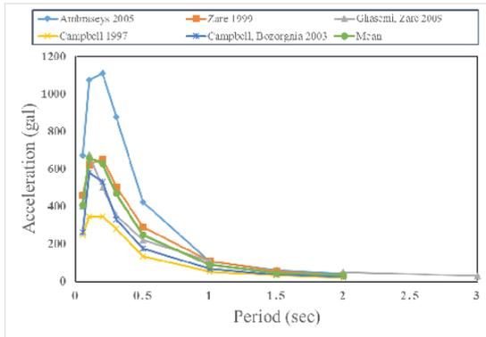
Figure 4. Uniform hazard spectra for center of Kangavar at bedrock with earthquake return period of 475 years
