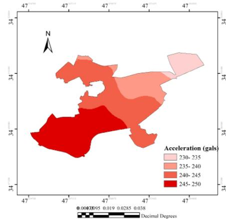
Figure 7. Micro-zonation of average horizontal  $S_a$  at 0.1 sec. and bedrock with earthquake return period of 475 years
