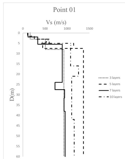
**Figure 14. Shear wave velocity profile for the point 1 from four initial model with 3, 5, 7, and 10 layers by inversion of H/V spectrum**
