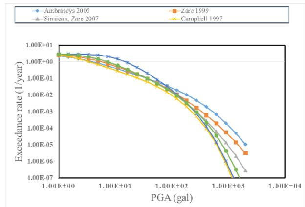
**Figure 3. Hazard curves for the center of Kangavar at bedrock**
