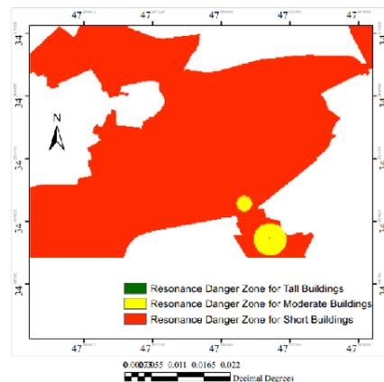
Figure 19. Construction guideline based on amplification hazard map for construction of filled frame buildings
