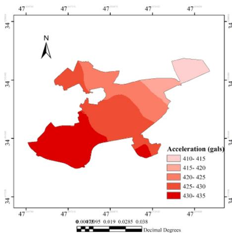
Figure 12. Micro-zonation of horizontal PGA at bedrock with earthquake return period of 2475 years
