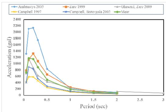
Figure 6. Uniform hazard spectra for center of Kangavar at bedrock with earthquake return period of 2475 years
