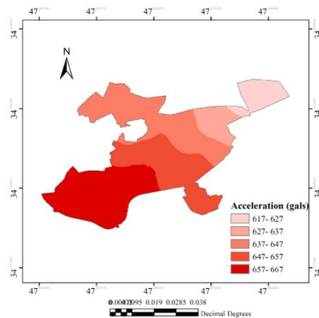
Figure 9. Micro-zonation of average horizontal  $S_a$  at 0.1 sec. and bedrock with earthquake return period of 2475 years
