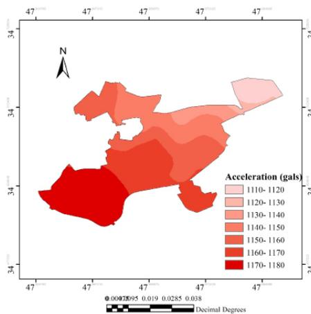
Figure 11. Micro-zonation of horizontal PGA at bedrock with earthquake return period of 975 years
