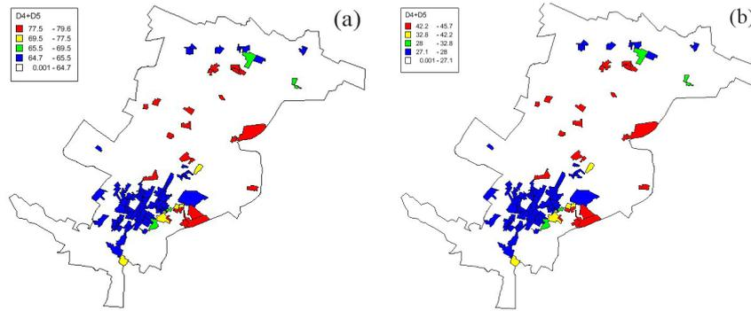
Figure 11. Percentage of damaged A1 buildings with level of D4+D5, (a) MCE, (b) DBE
