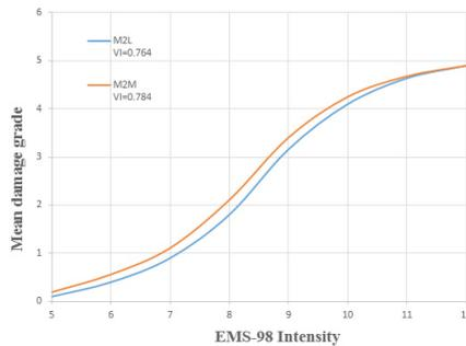
Figure 5. Average damage grade in terms of EMS-98 for brick wall and steel beam (M2) [10]
