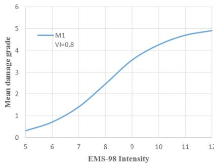
Figure 4. Average damage grade in terms of EMS-98 for brick wall and wooden beam (M1) [10]
