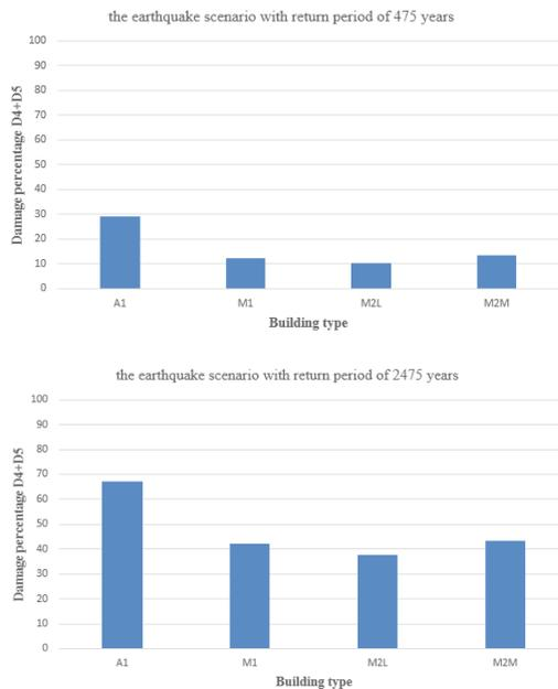
Figure 12. Percentage of damaged buildings with level of D4+D5, (a) DBE, (b) MCE
