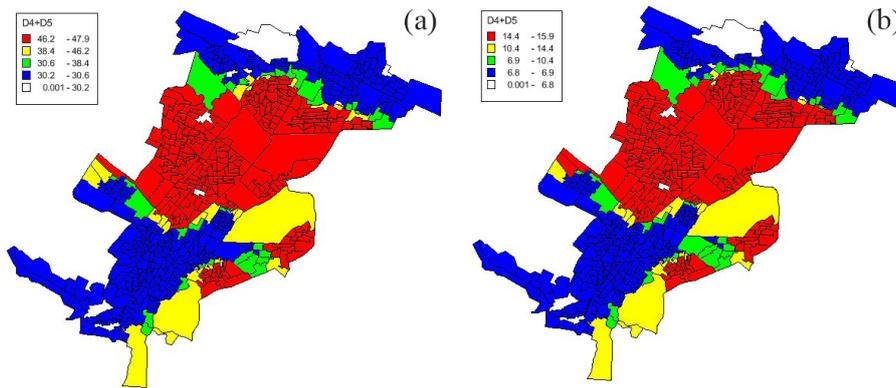
Figure 9. Percentage of damaged M2L buildings with level of D4+D5, (a) MCE, (b) DBE
