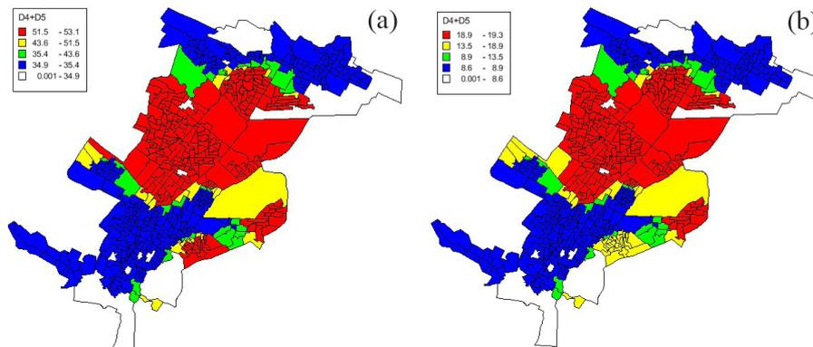
Figure 10. Percentage of damaged M2M buildings with level of D4+D5, (a) MCE, (b) DBE
