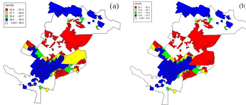
Figure 8. Percentage of damaged M1 buildings with level of D4+D5, (a) MCE, (b) DBE
