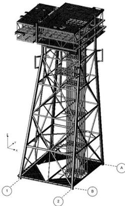
Figure 1. Perspective plot of SPD12 jacket platform [14]
