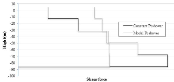
Figure 11. Comparison of shear force in each story due to loading pattern
