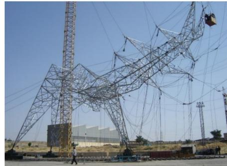
(b) Typical failure of lattice transmission tower in type test
