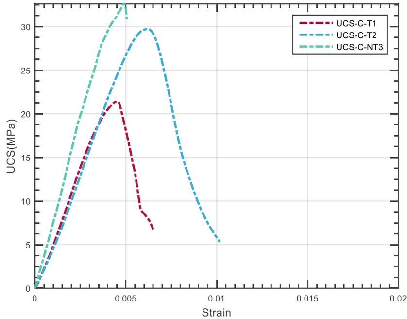
Fig. 3. UCS - 25°C temperature - Concrete
