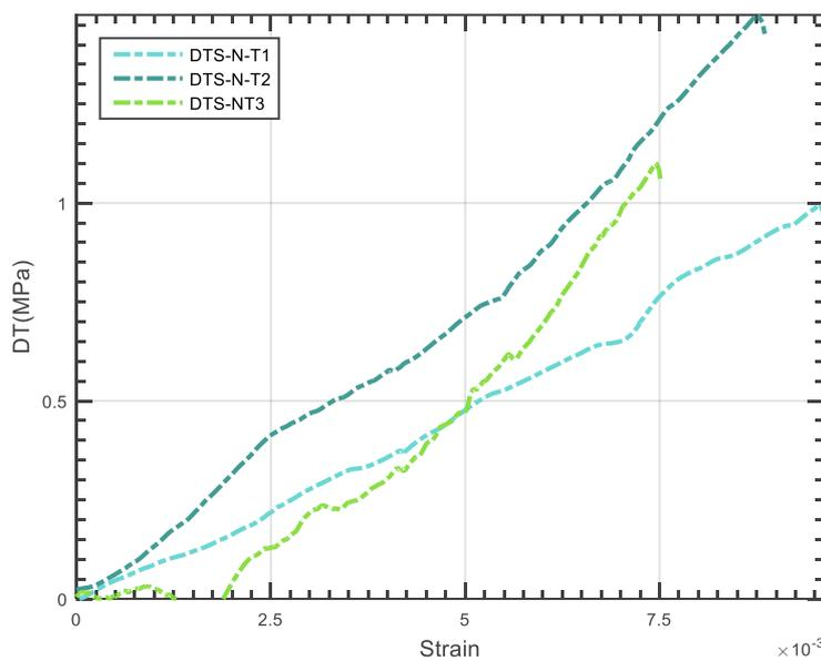
Fig. 6. Direct tensile strength change related to 350°C temperature – Marble
