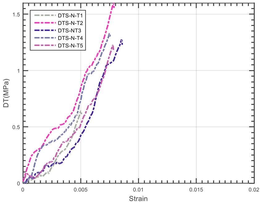
Fig. 10. Direct tensile strength change related to 350°C temperature –for concrete mixture design
