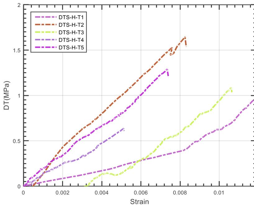
Fig. 8. Direct tensile strength change related to 350°C temperature – Travertine
