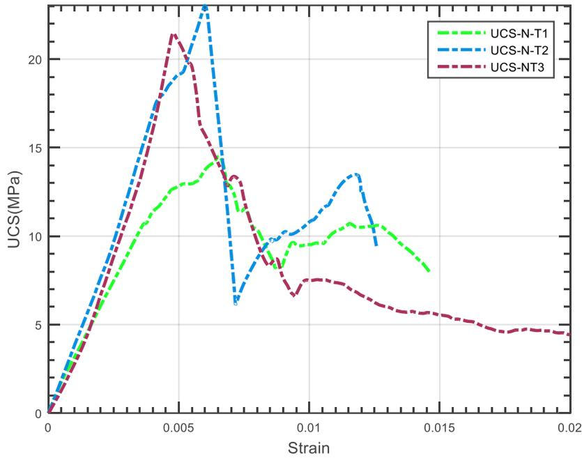
Fig. 1. UCS - 25°C temperature – Travertine
