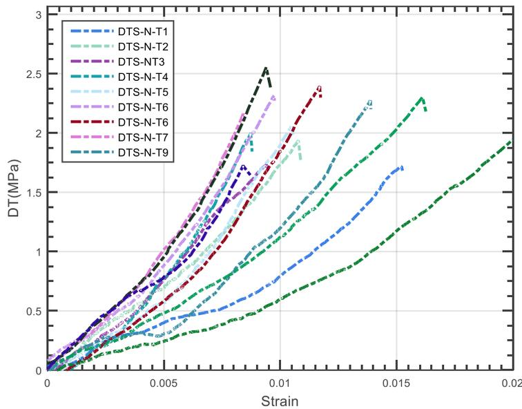
Fig. 5. Direct tensile strength change related to 25°C temperature – Marble
