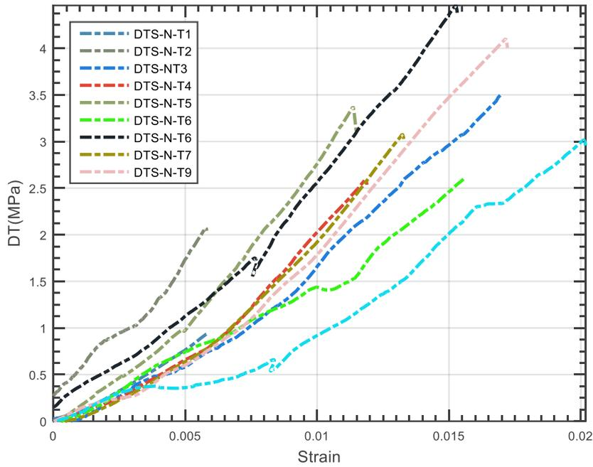
Fig. 7. Direct tensile strength change related to 25°C temperature – Travertine
