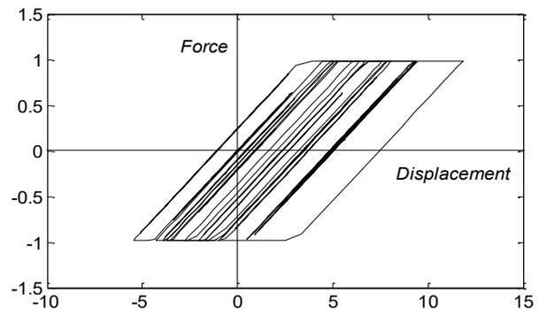
Figure 12. Force-displacement response of elastic-perfectly plastic SDOF
