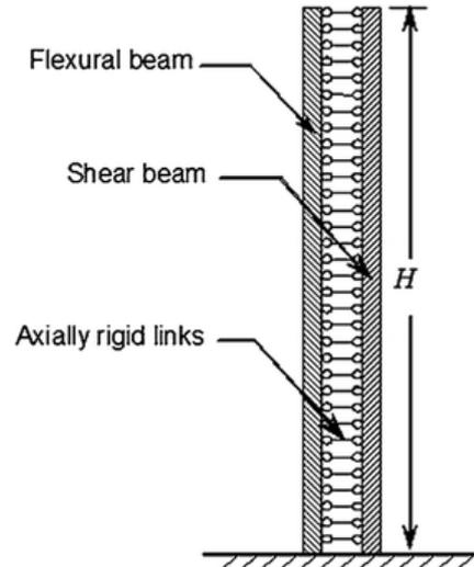
Fig. 9. Simplified model for assessing building response (Miranda and Akkar [14]).
