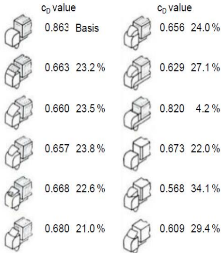
Fig.1. effect of extensions on drag coefficient (Welfers, Ginsberg et al. 2011)
