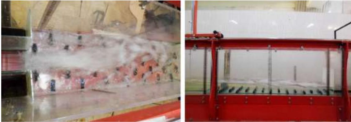
Fig. 3. View of S-jump on the rough bed
