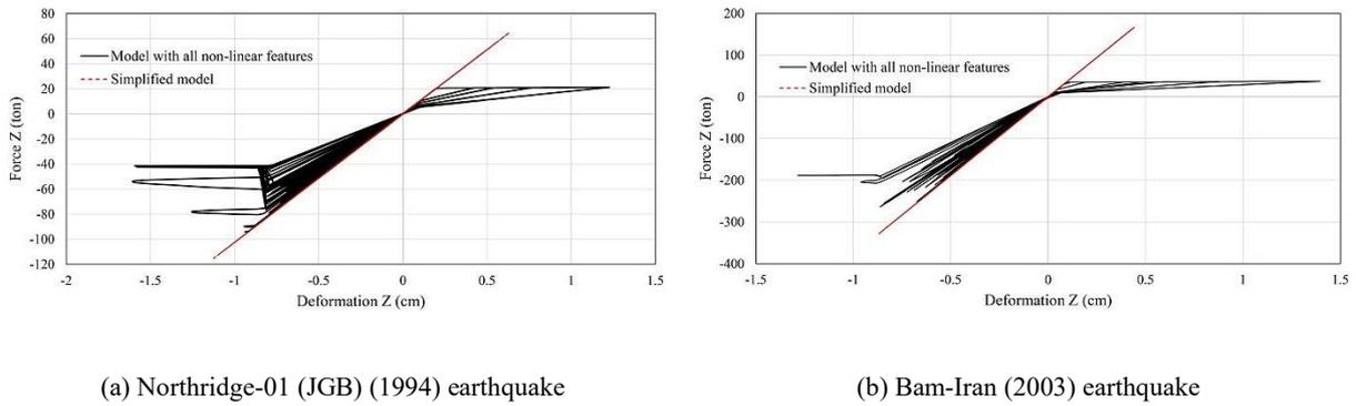
Fig. 7. Axial force-deformation curves including and excluding consideration of the main aspects of LRB modeling
