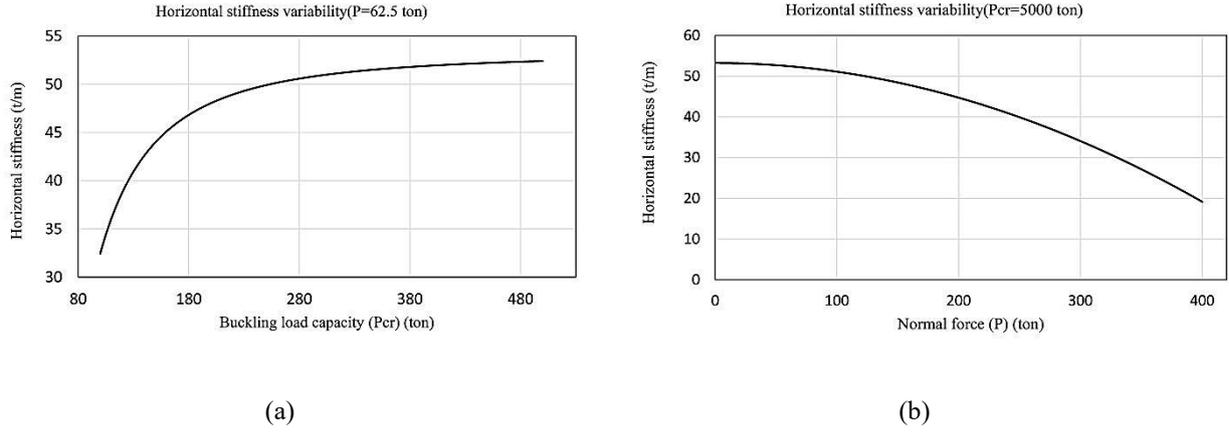
Fig. 5. Shear stiffness variability of the LR isolator as a function of the (a) applied normal force (P) and (b) buckling load capacity changes ( $P'_{cr}$ )
