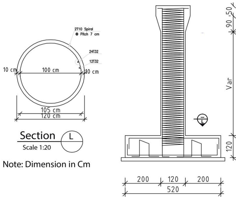
Fig. 2. Bridge circular column cross sections and reinforcing detail
