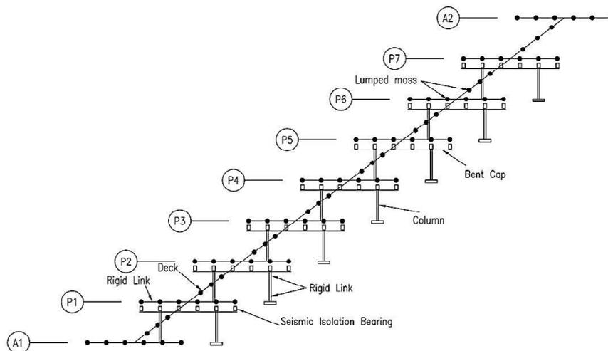
Fig. 3. Model of seismically isolated bridge in OpenSees
