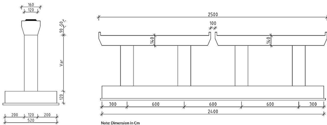
Fig.1. Bridge cross section and Pier details
