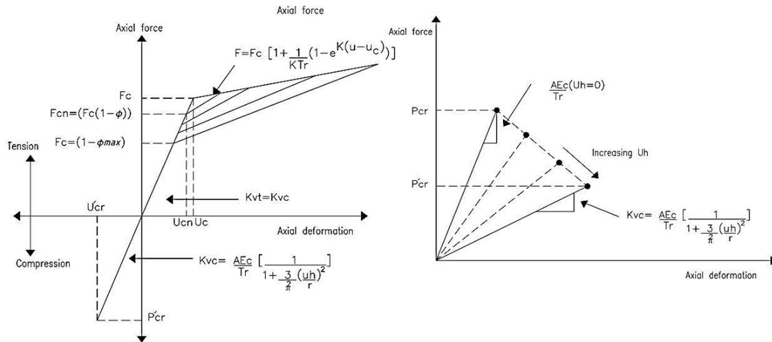
**Fig. 4. Mathematical model of elastomeric bearings behavior in axial direction [2]**
