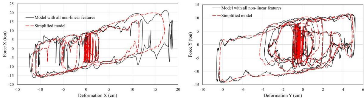
Fig. 9. Shear force-deformation curves in X and Y directions including and excluding consideration of the main aspects of LRB modeling for the Northridge (1994) earthquake.
