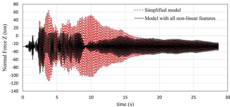
Fig. 8. Normal force time history of LR isolator including and excluding consideration of the main aspects of LRB modeling under the Northridge-01 (JGB) (1994) earthquake.
