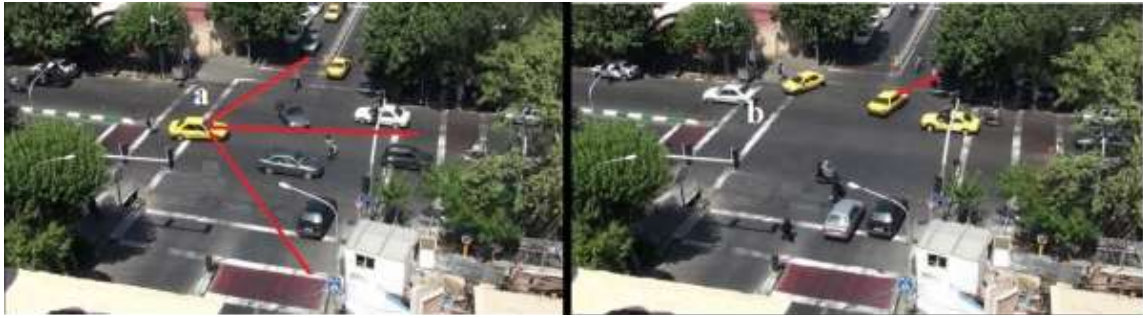
Fig. 5. A conflict between a left-turning vehicle and a pedestrian
