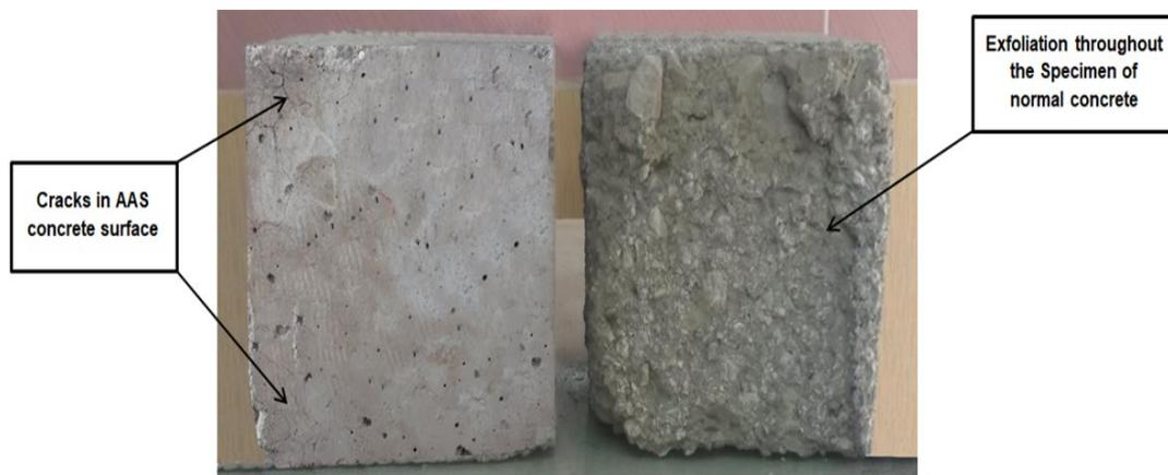
Fig. 6. Surface textures of concrete at 800 °C.
