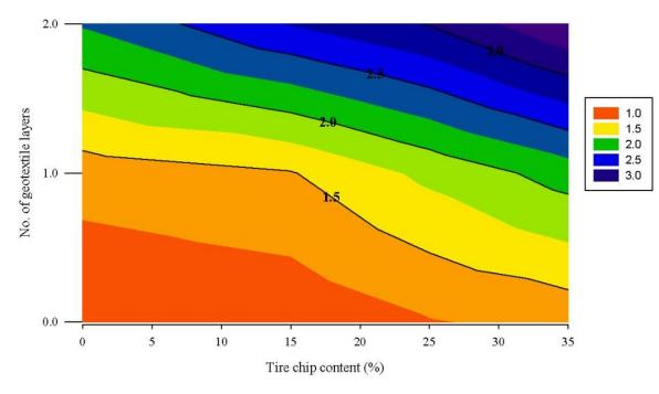
Fig. 16. Strength ratio contours at strain level 18% under confining pressure of 50 Pa
