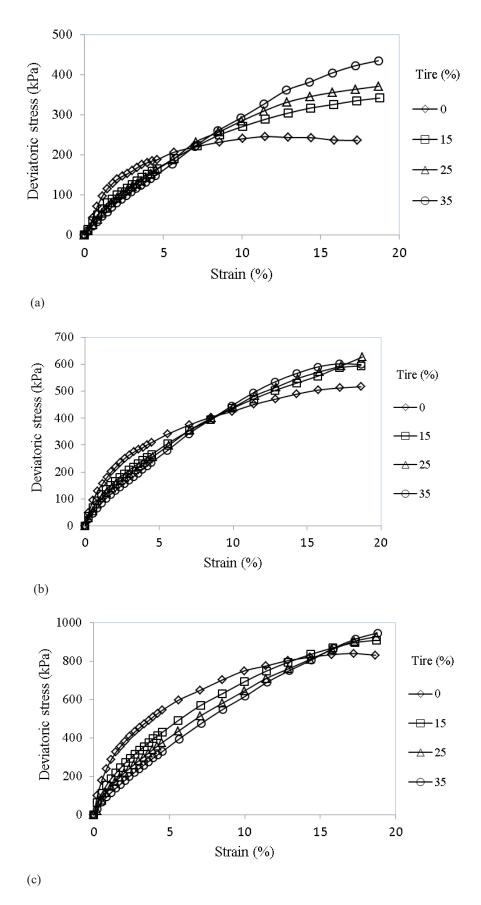
Fig. 8. Stress-axial strain curves for tire chip-reinforced sand with two layers of geotextile under various confining pressure (a) 50 kPa; (b) 100 kPa; and (c) 200 kPa
