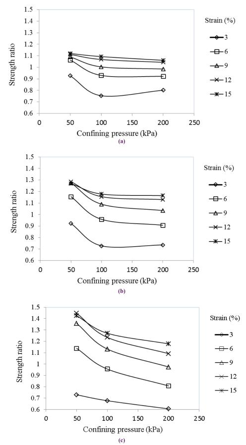
Fig. 14. Strength ratio values versus confining pressure at different strain levels and for various tire chip contents: (a) 15%; (b) 25% and (c) 35%
