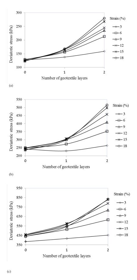
Fig. 9. Deviatoric stress values versus number of reinforcement at different strain levels under various confining pressure (a) 50 kPa; (b) 100 kPa and (c) 200 kPa
