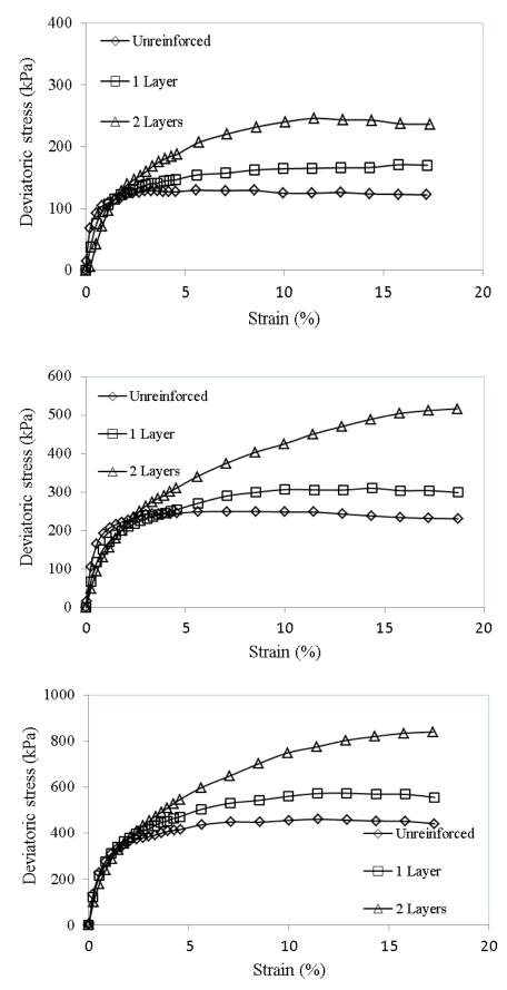
Fig. 5. Stress-axial strain curves for reinforced and unreinforced sand under various contining pressure (a) 50 kPa; (b) 100 kPa; and (c) 200 kPa
