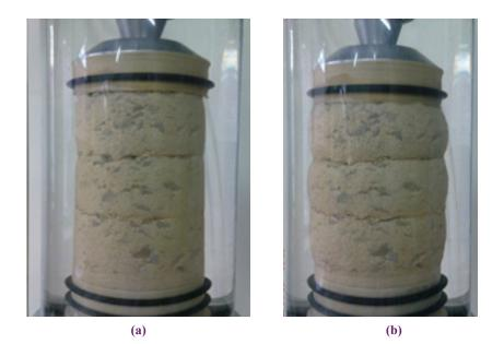
Fig. 4. Sample of the sand-tire chips mixture with two layers of geotextile: a) before testing and b) after testing
