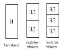
Fig. 3. Geotextile arrangements for triaxial tests
