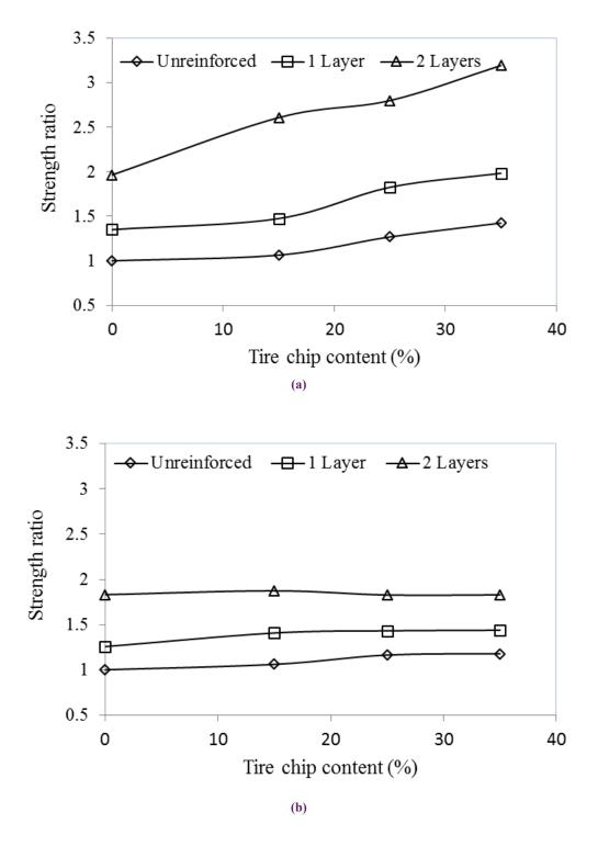
Fig. 15. Strength ratio values versus tire chip content for various number of reinforcement at strain level 15% under confining pressure of: (a) 50 kPa and (b) 200 kPa
