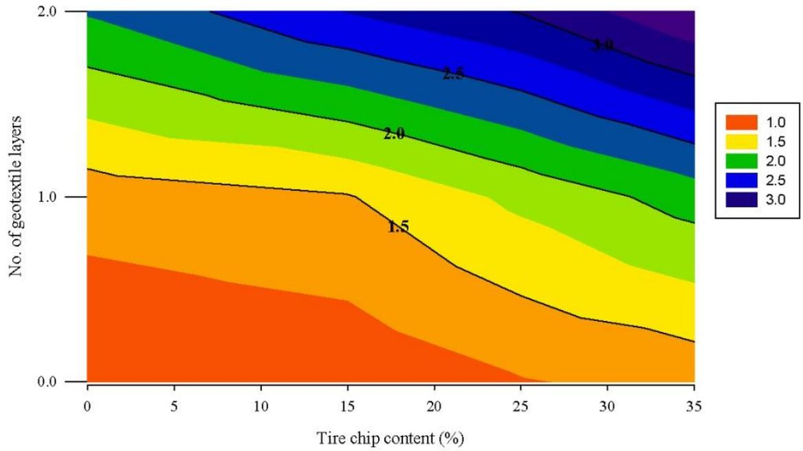
Fig. 16. Strength ratio contours at strain level 18% under confining pressure of 50 Pa
