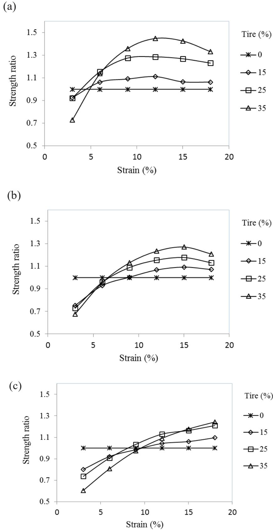
**Fig. 10. Strength ratio values versus number of reinforcement at different strain levels under various confining pressure (a) 50 kPa; (b) 100 kPa and (c) 200 kPa**
