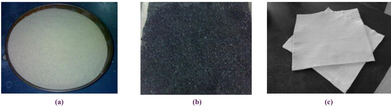
Fig. 2. Materials: a) sand, b) tire chips, and c) geotextile specimen
