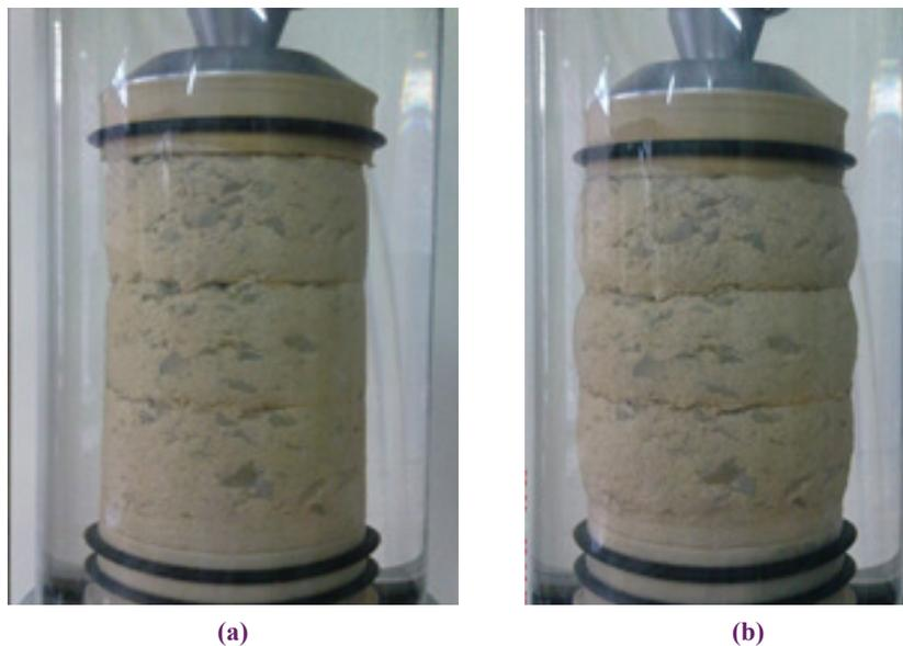
**Fig. 4. Sample of the sand-tire chips mixture with two layers of geotextile: a) before testing and b) after testing**
