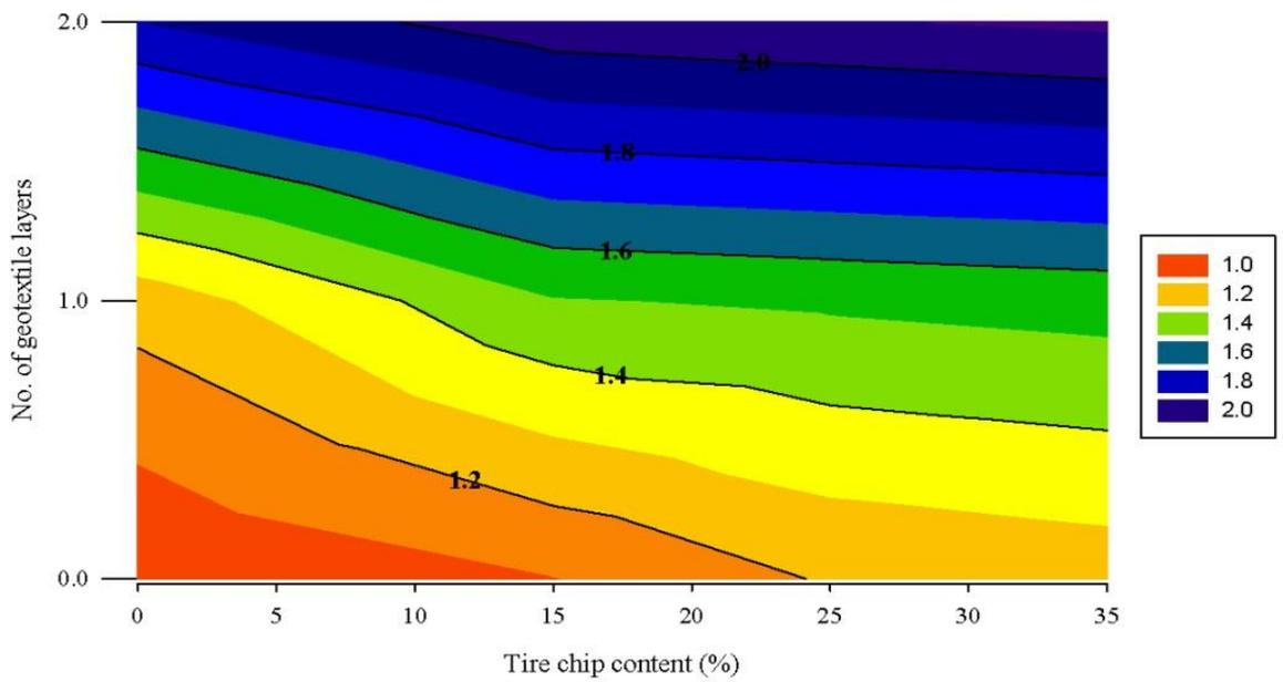
Fig. 17. Strength ratio contours at strain level 18% under confining pressure of 200 Pa
