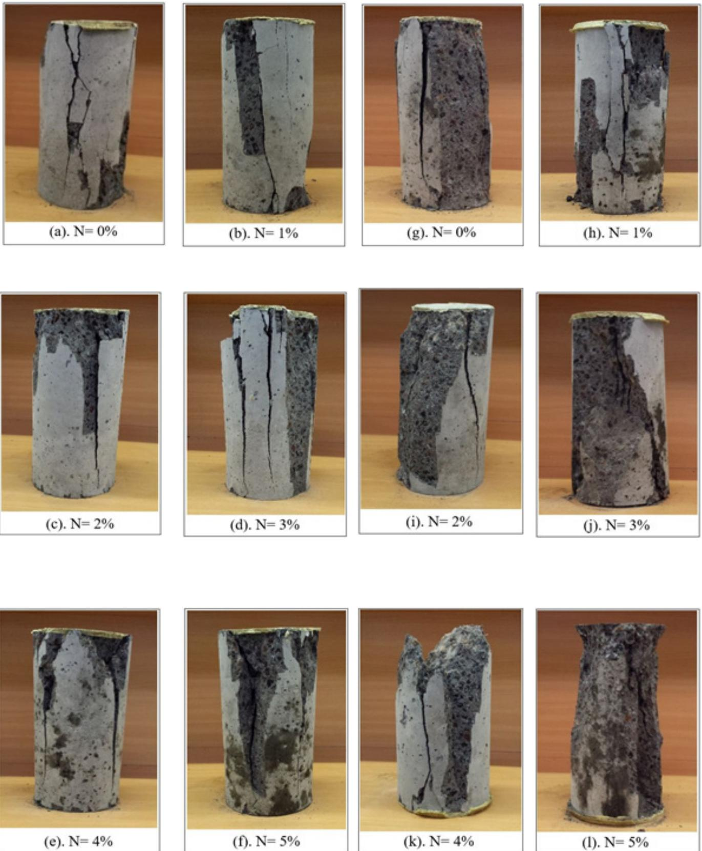
Fig. 10. Failure mode of NS-incorporated LWAC under (a–f) monotonic and (g–l) cyclic compressive loading
