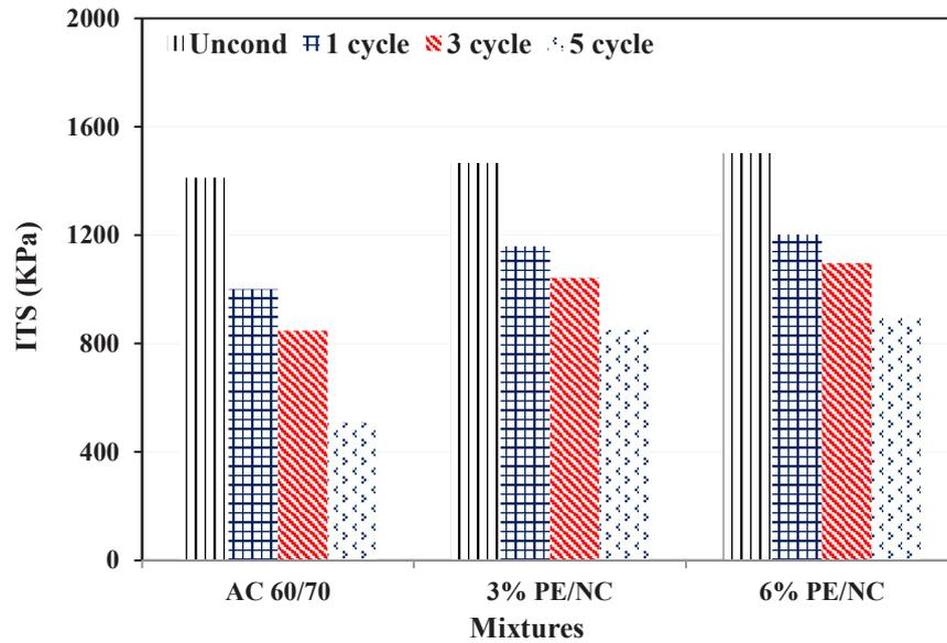
Fig. 5. ITS for mixtures made with granite aggregate with and without PE/NC.
