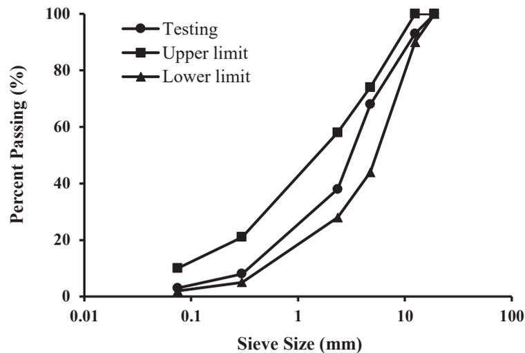
Fig. 1. Three limits of aggregates gradation.
