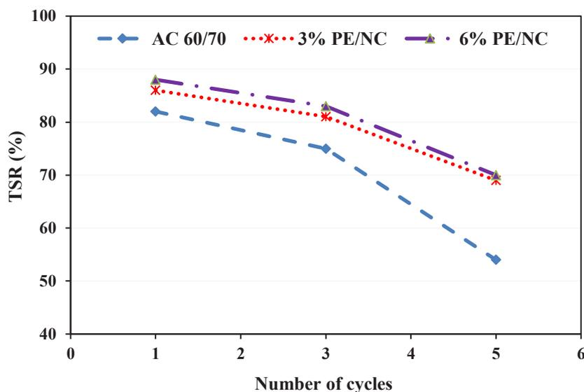
Fig. 8. Effects of PE/NC and freeze-thaw cycles on TSR in mixtures made with limestone aggregate.
