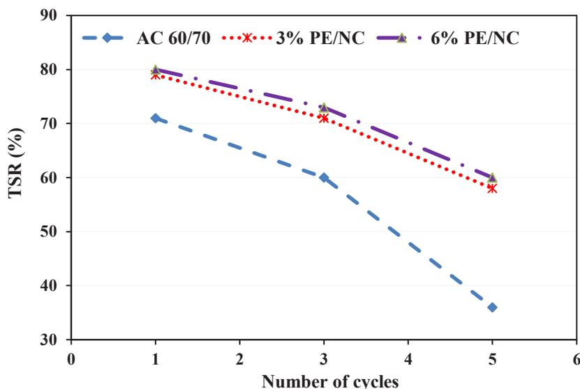
Fig. 7. Effects of PE/NC and freeze-thaw cycles on TSR in mixtures made with granite aggregate.
