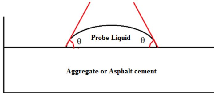
**Fig. 2. Contact angles measured in the sessile drop method.**
