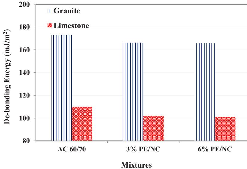
**Fig. 4. Adhesion surface free energy of different mixtures at wet condition (De-bonding energy).**
