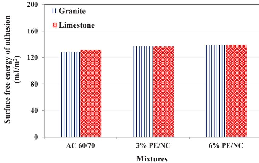
Fig. 3. Adhesion surface free energy of different mixtures at dry condition.
