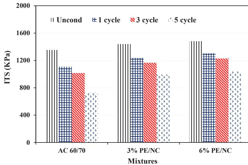
Fig. 6. ITS for mixtures made with limestone aggregate with and without PE/NC.
