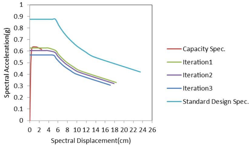
Fig. 14. Performance point according to the capacity spectrum procedure (ADRS).
