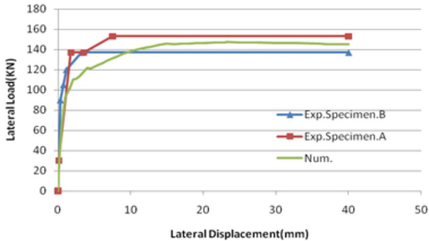
**Fig. 3. Comparison between the capacity curve of experimental and numerical models [6, 19].**
