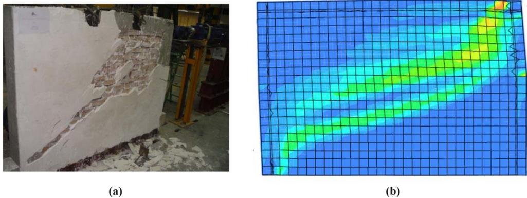
**Fig. 4. Comparison between fracture mechanism of the experimental and numerical models; (a) Experimental model, (b) Numerical model [6, 19].**
