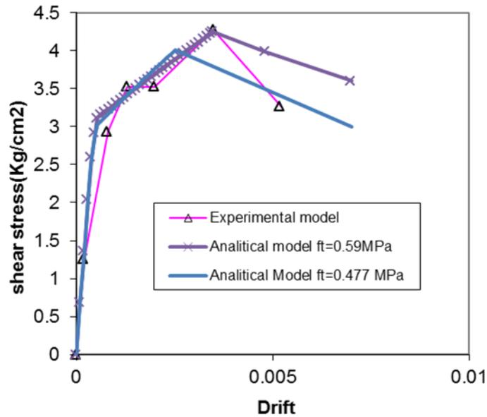
Fig. 8. The comparison of the capacity curve between experimental and numerical models [6, 26].
