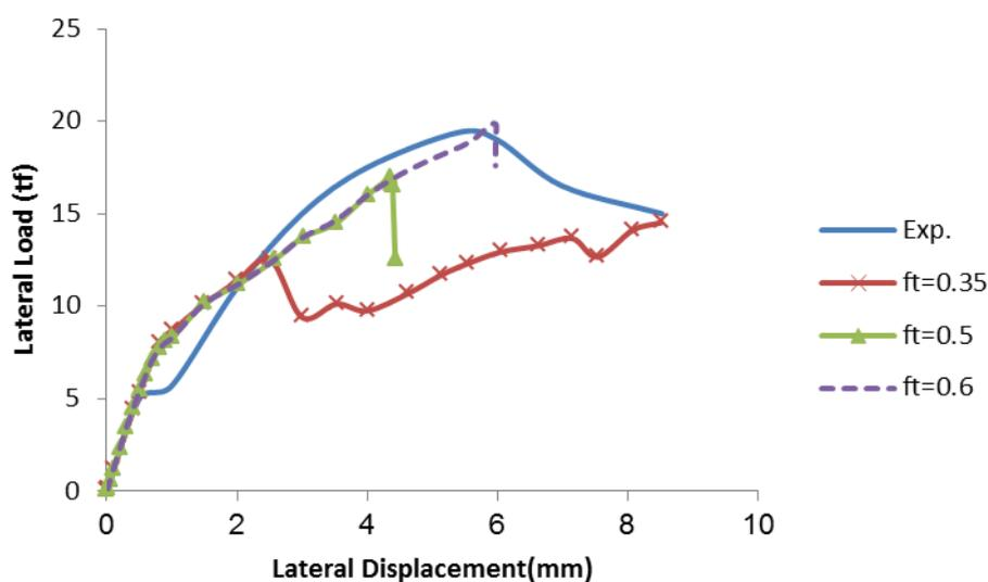
**Fig. 5. Comparison between the capacity curve of experimental and numerical models [6, 23].**
