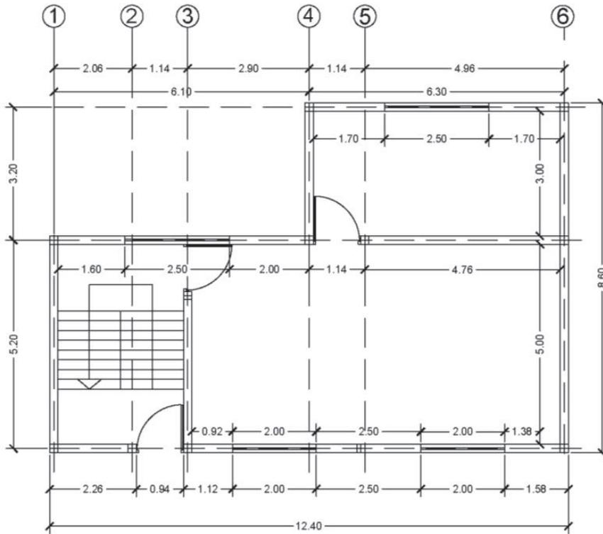
Fig. 11. Plan with 82 m<sup>2</sup> (model 2).
