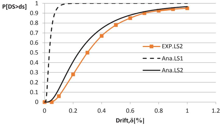
Fig. 7. The drift-based fragility curves correspond to the maximum strength (LS2) and the elastic limit strength (LS1) for CMWs [5, 6].
