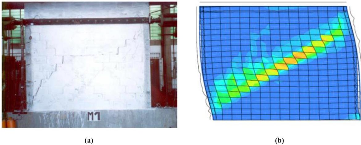
**Fig. 6. Comparison between fracture mechanism of the experimental and numerical models; (a) Experimental model, (b) Numerical model [6, 23].**
