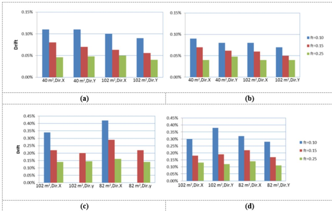
**Fig. 15. Drift angle data for prototype models, a) one story with a thickness of walls 22 cm, b) one story with a thickness of walls 35 cm, c) two-story with a thickness of walls 22 cm, and d) two-story with a thickness of walls 35 cm.**
