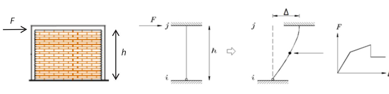
Fig. 2. Proposed Macro and analytical model for confined masonry wall [6].
