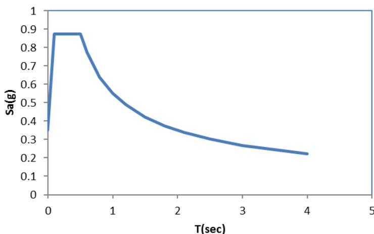
**Fig. 1. Standard design spectrum (Standard No.2800) [16].**
