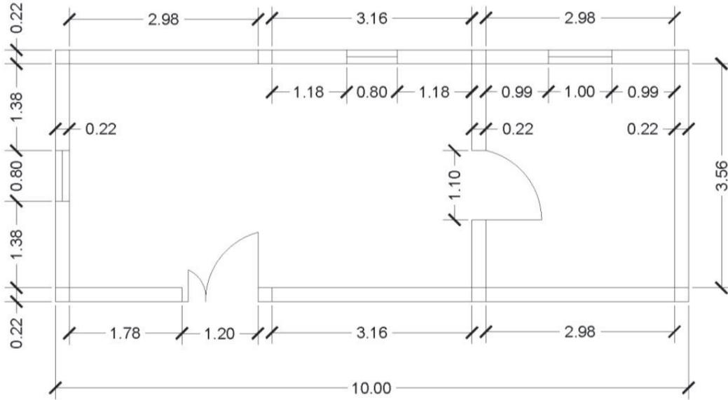
Fig. 10. Plan with 40 m<sup>2</sup> (model 1) [9].
