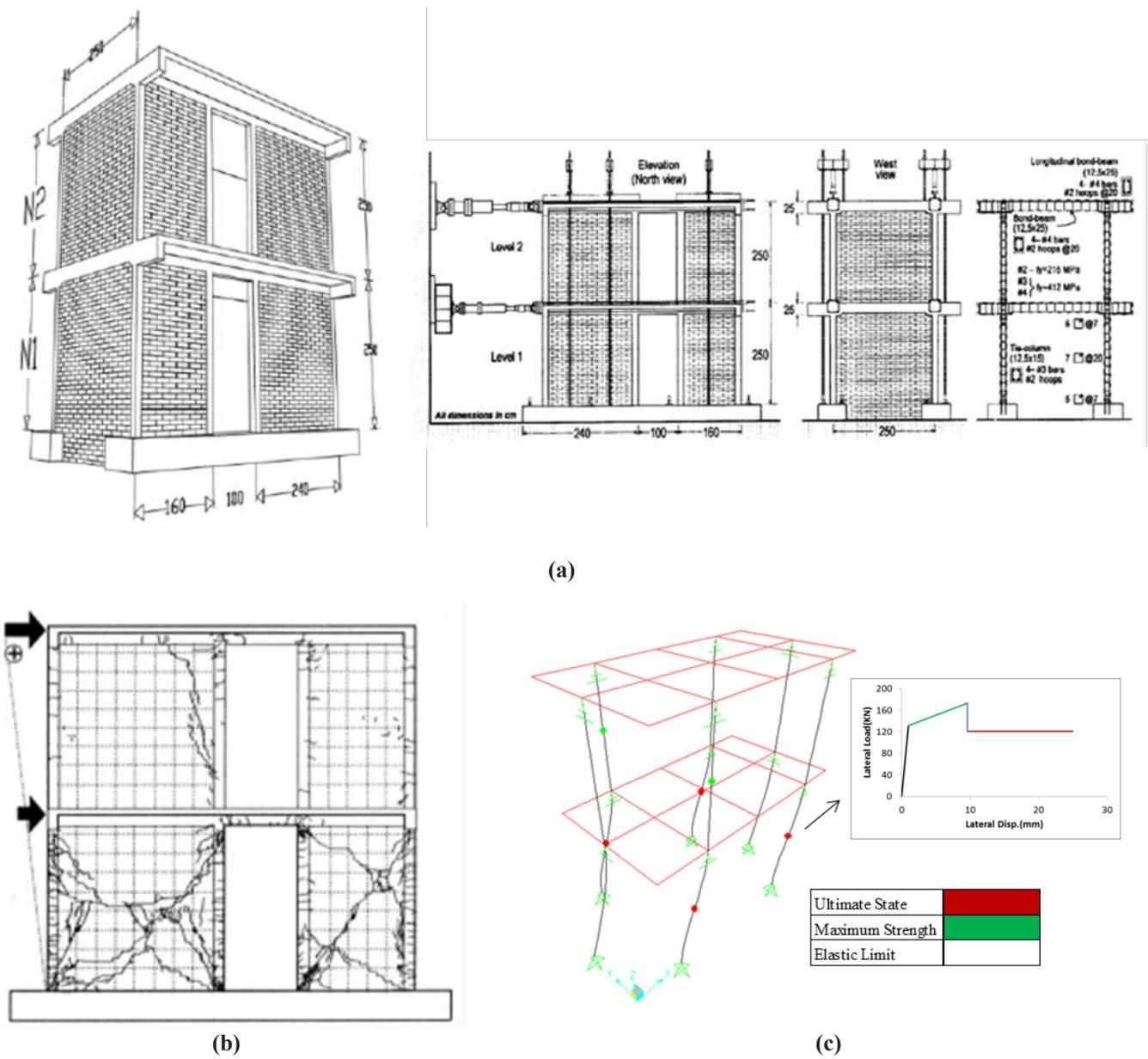
Fig. 9. The comparison of damage mechanism between experimental and numerical study; (a) 3-D experimental model [26], (b) Damage status in the experimental model [26], and (c) Damage status and distribution of plastic hinge by numerical model [6]
