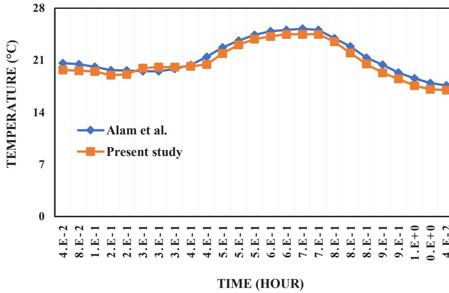
Fig. 7. Indoor air temperature of the single zone building.
