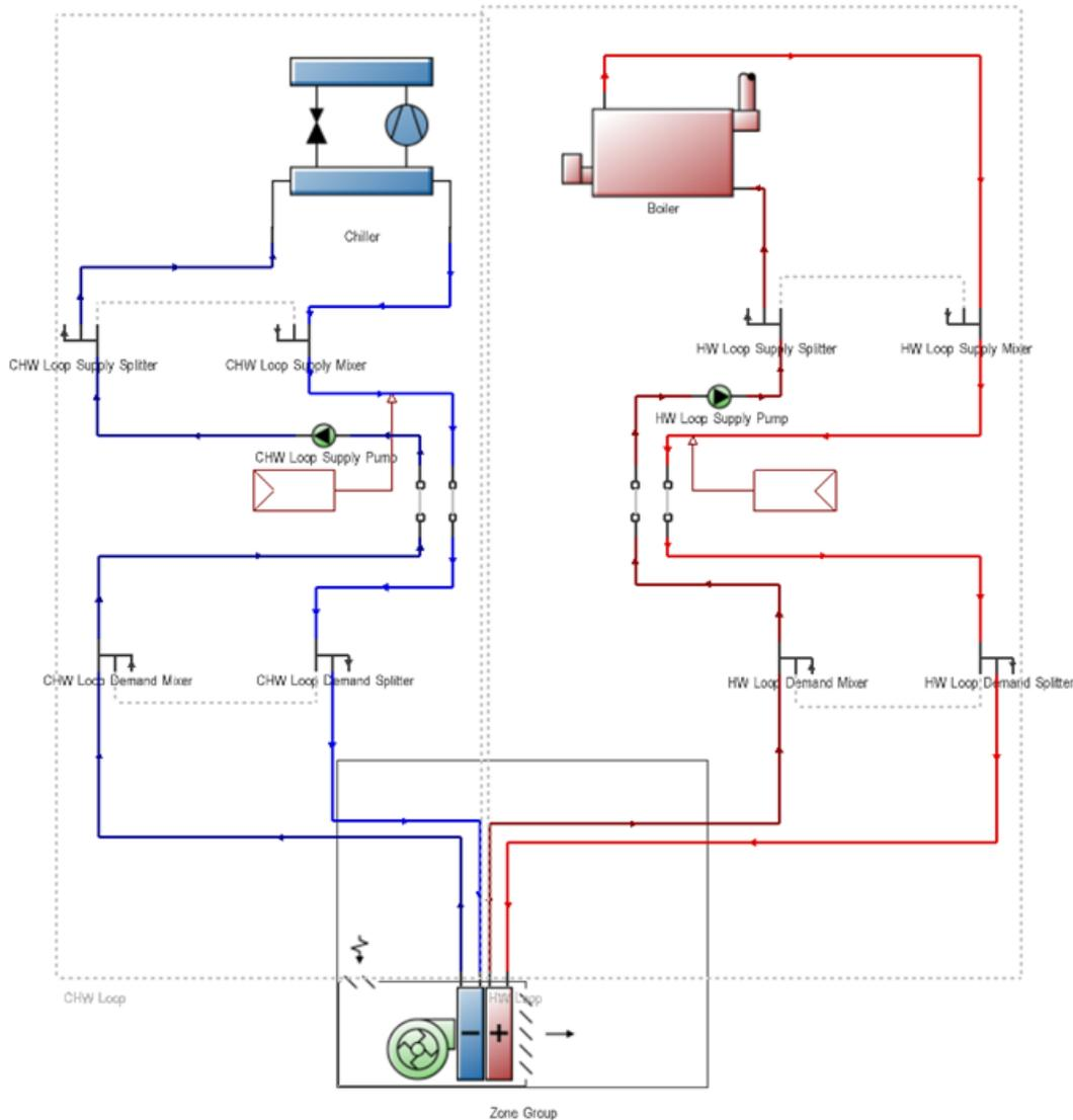
**Fig. 6. schematic of FCU system.**
