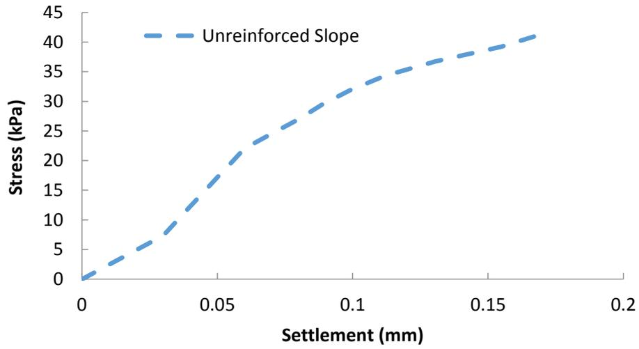
Fig. 4. The load-settlement diagram for footing located on unreinforced sandy soil slope
