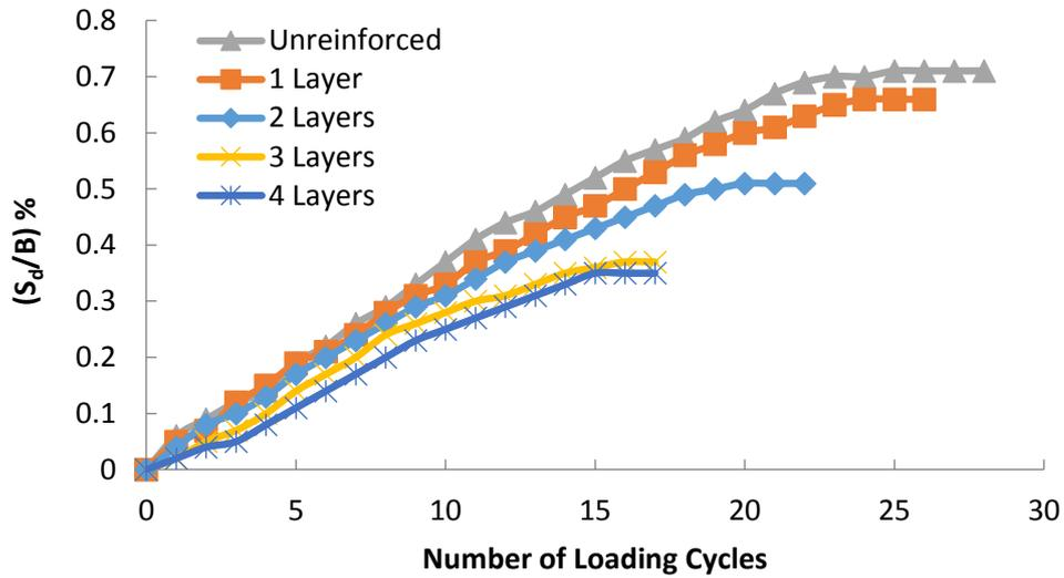
Fig. 7. Variations of  $(S_d/B)$  with the number of loading cycles when  $q_d=0.50q_u$  (geogrid).
