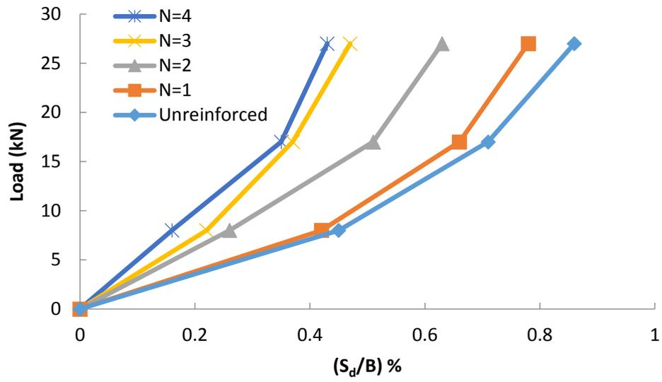
Fig. 15. Variations of load with  $(S_d/B)$  (geogrid).
