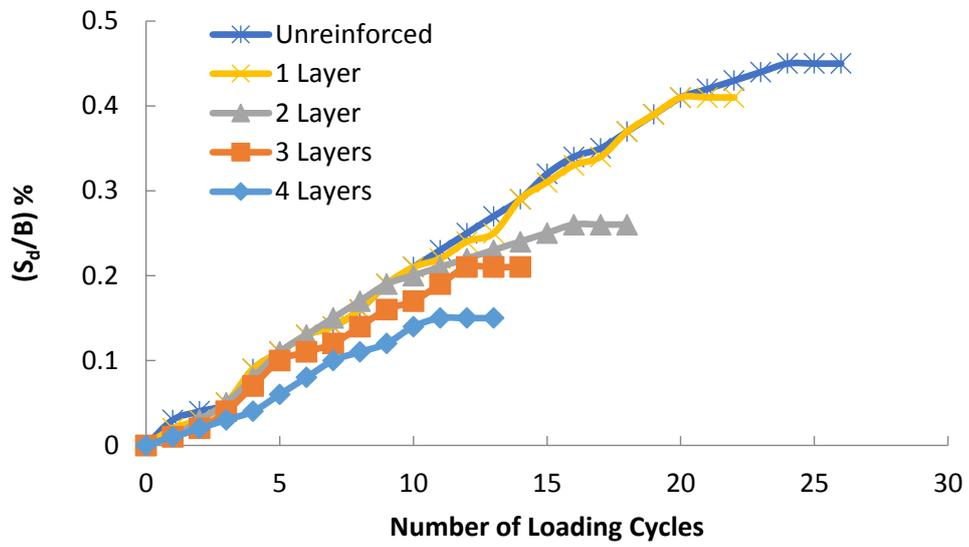
Fig. 11. Variations of  $(S_d/B)$  with the number of loading cycles when  $q_d=0.25q_u$  (grid anchor).
