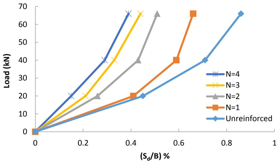
Fig. 16. Variations of load with  $(S_d/B)$  (grid anchor).
