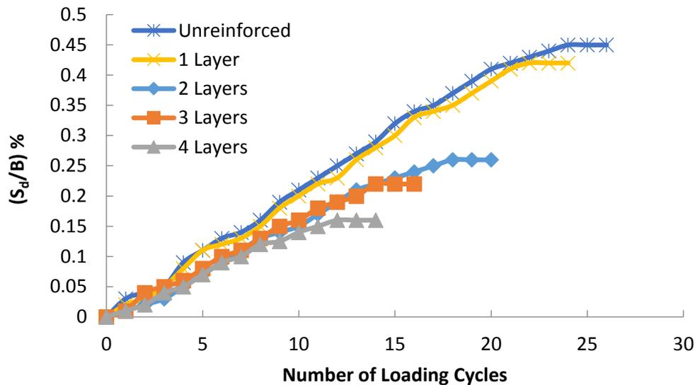
Fig. 8. Variations of  $(S_d/B)$  with the number of loading cycles when  $q_d=0.25q_u$  (geogrid).
