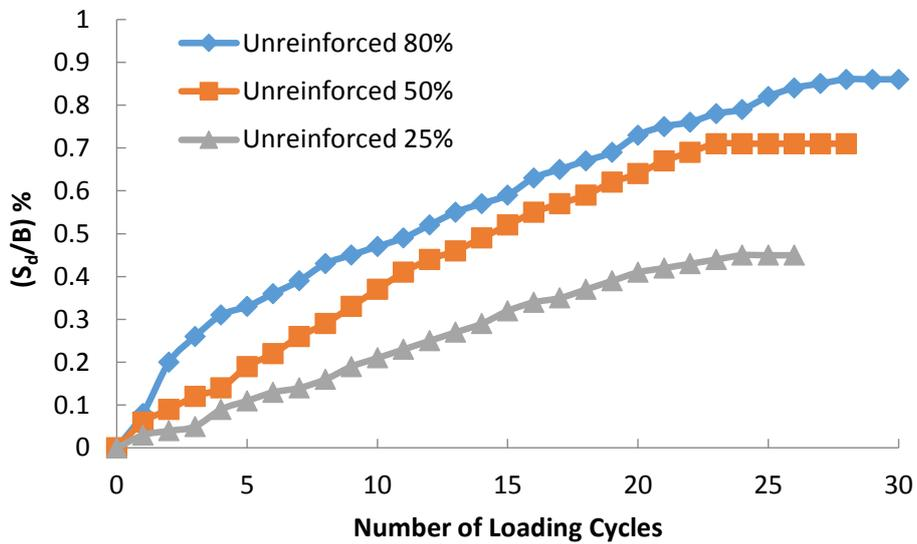
Fig. 5. Variations of  $(S_d/B)$  with the number of loading cycles for Series CS tests.
