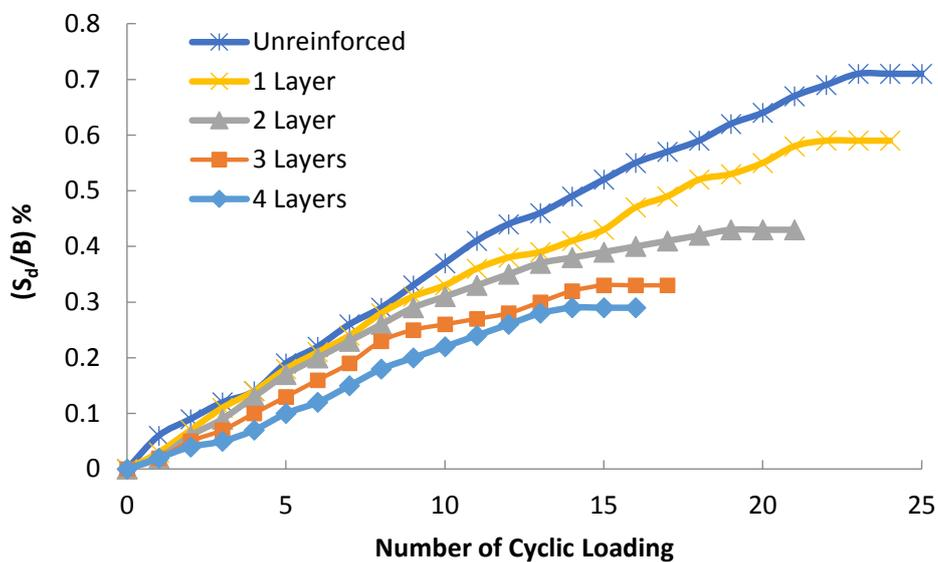
Fig. 10. Variations of  $(S_d/B)$  with the number of loading cycles for when  $q_d=0.50q_u$  (grid anchor).
