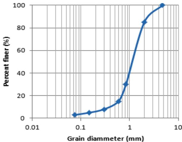
Fig. 2. The grading curve of the used sandy soil.
