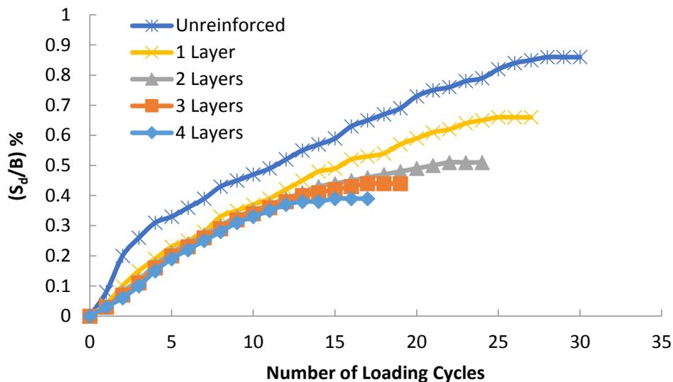
Fig. 9. Variations of  $(S_d/B)$  with the number of loading cycles when  $q_d=0.80q_u$  (grid anchor).
