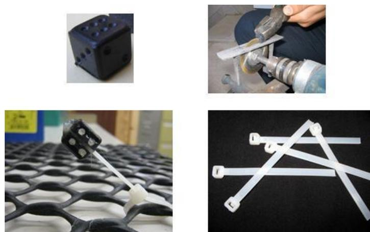
**Fig. 3. Grid-Anchor component and production process.**
