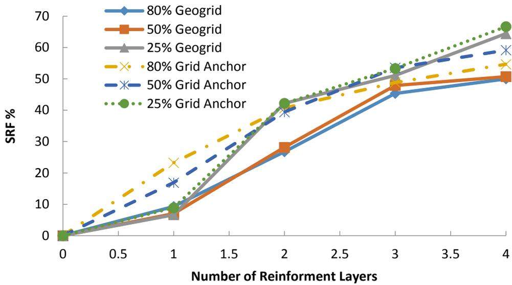
Fig. 12. Variations of SRF with the number of reinforcement layers.
