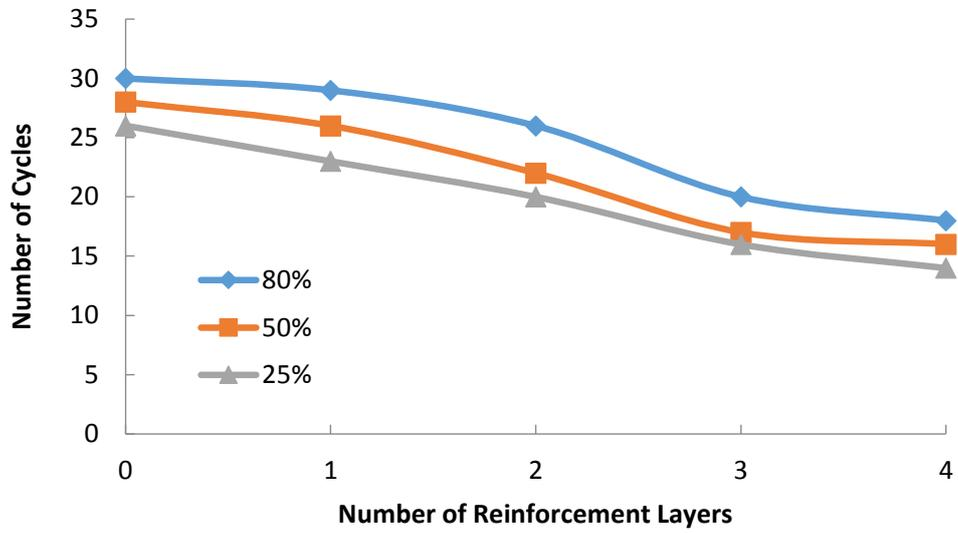
Fig. 13. Variations of SRF with the number of reinforcement layers (geogrid).
