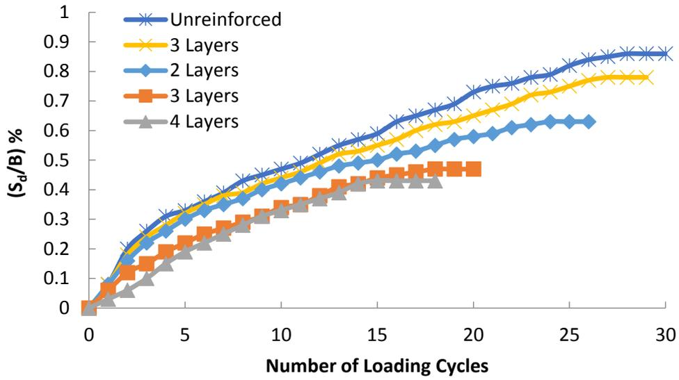
Fig. 6. Variations of  $(S_d/B)$  with the number of loading cycles when  $q_d=0.80q_u$  (geogrid).
