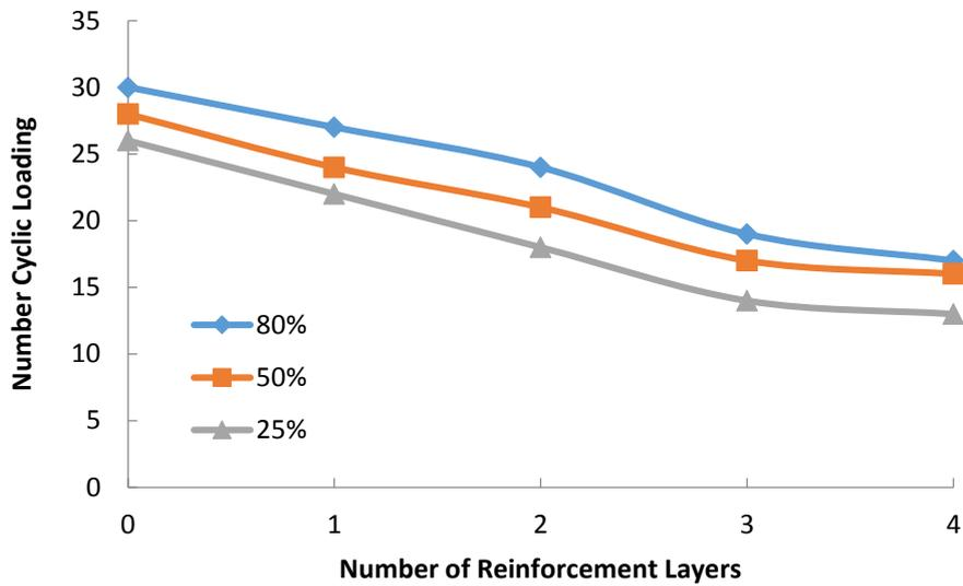
Fig. 14. Variations of SRF with the number of reinforcement layers (grid anchor).
