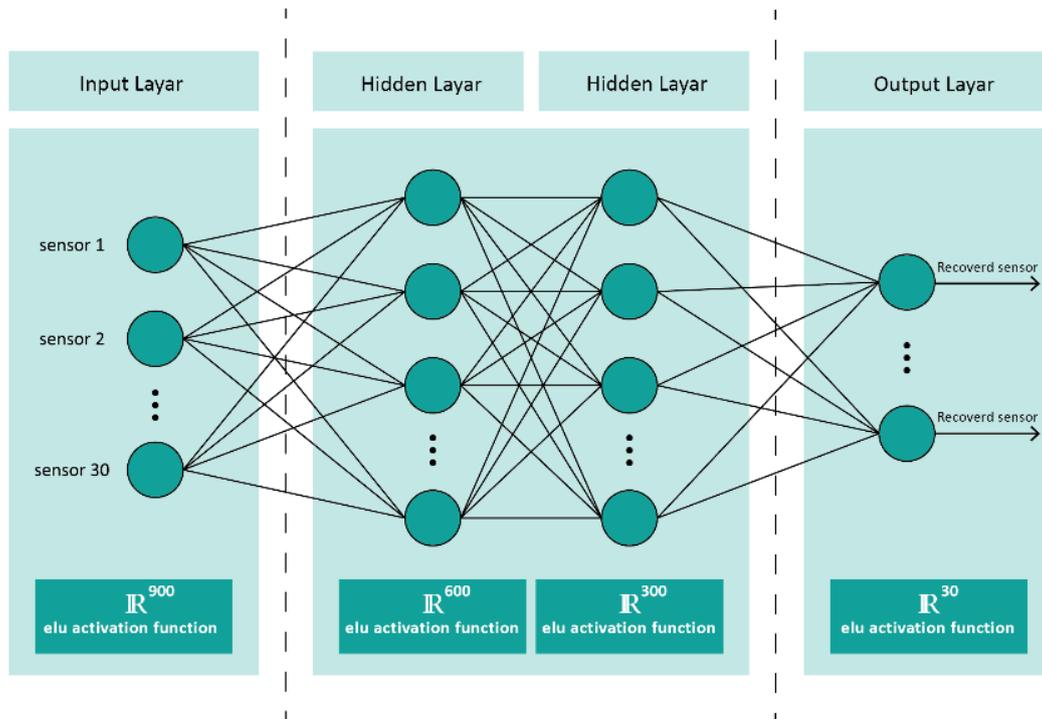
**Fig. 6. The proposed NN architecture for the recovery of Alamosa Canyon Bridge.**
