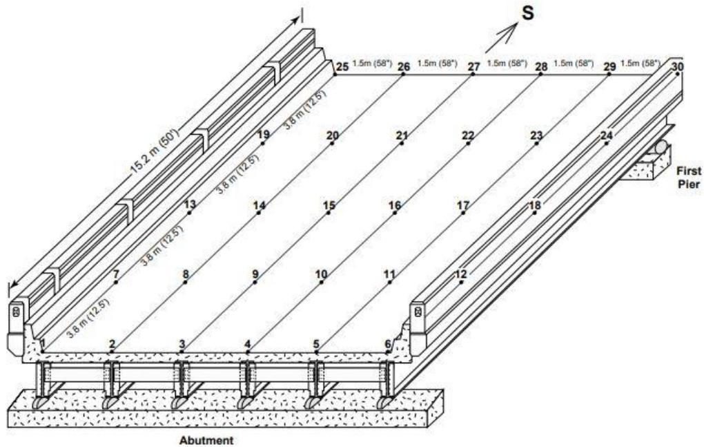
Fig. 3. Schematic location of accelerometers in Farrar’s experiment [36].
