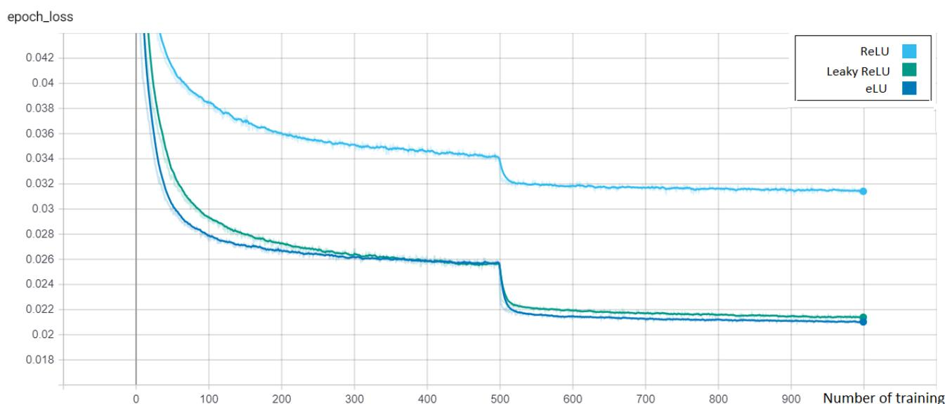
**Fig. 13. Convergence curve of three common activation functions for model (a)**
