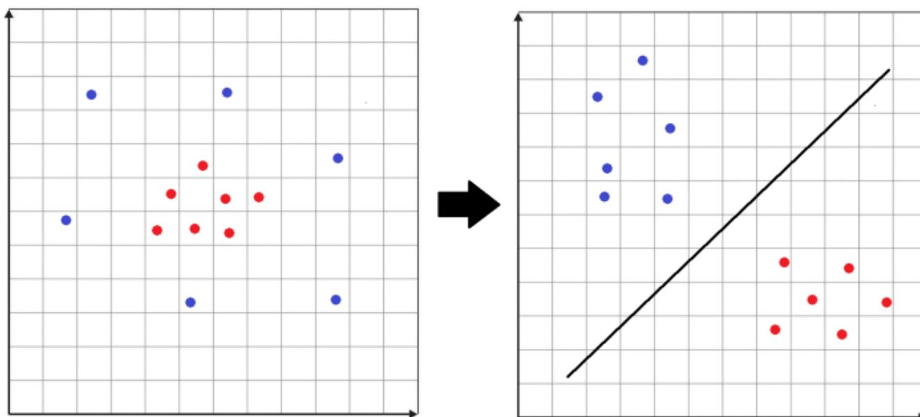
Fig. 4. Mapping data into separable space by the Kernel function [52].
