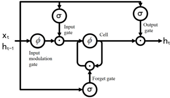
Fig. 2. The architecture of an LSTM network [37].
