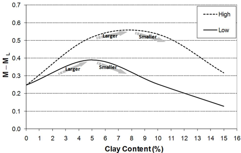
**Fig. 11. Variation of instability zone for mixtures of sand with low- and high-plasticity clays.**
