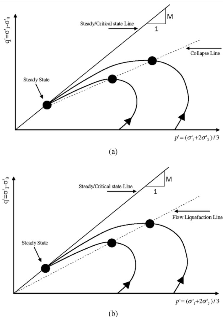
**Fig. 1. Schematic diagram of (a) the collapse line concept and (b) the flow liquefaction line concept.**
