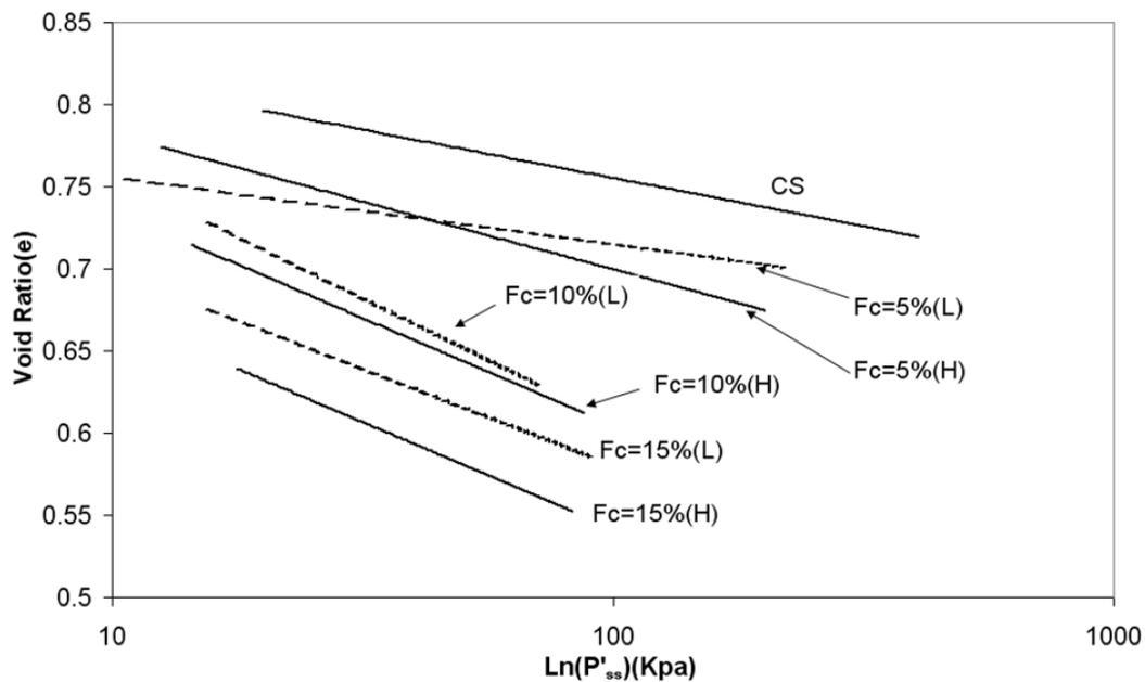
**Fig. 14. Steady-state lines for sand mixtures with different types of clayey materials.**
