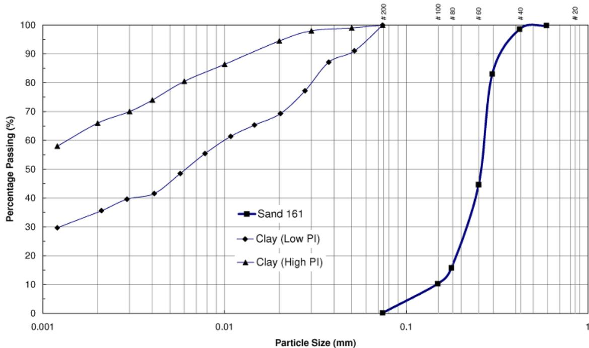
Fig. 2. The grain size analysis (Sand 161, Mashhad clay (Low PI), Gazvin clay (High PI)).
