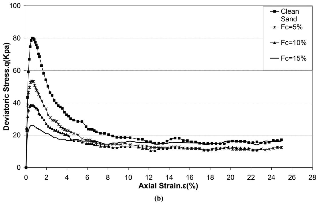
Fig. 5. Stress-strain variations for different mixtures of sand and clay. a) 1.45-100-L. b) 1.45-100-H
