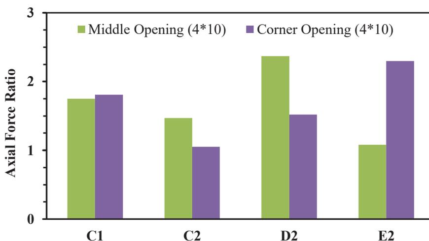
Fig. 18. Effect of the opening location on the openings of dimension (4\*10 m).
