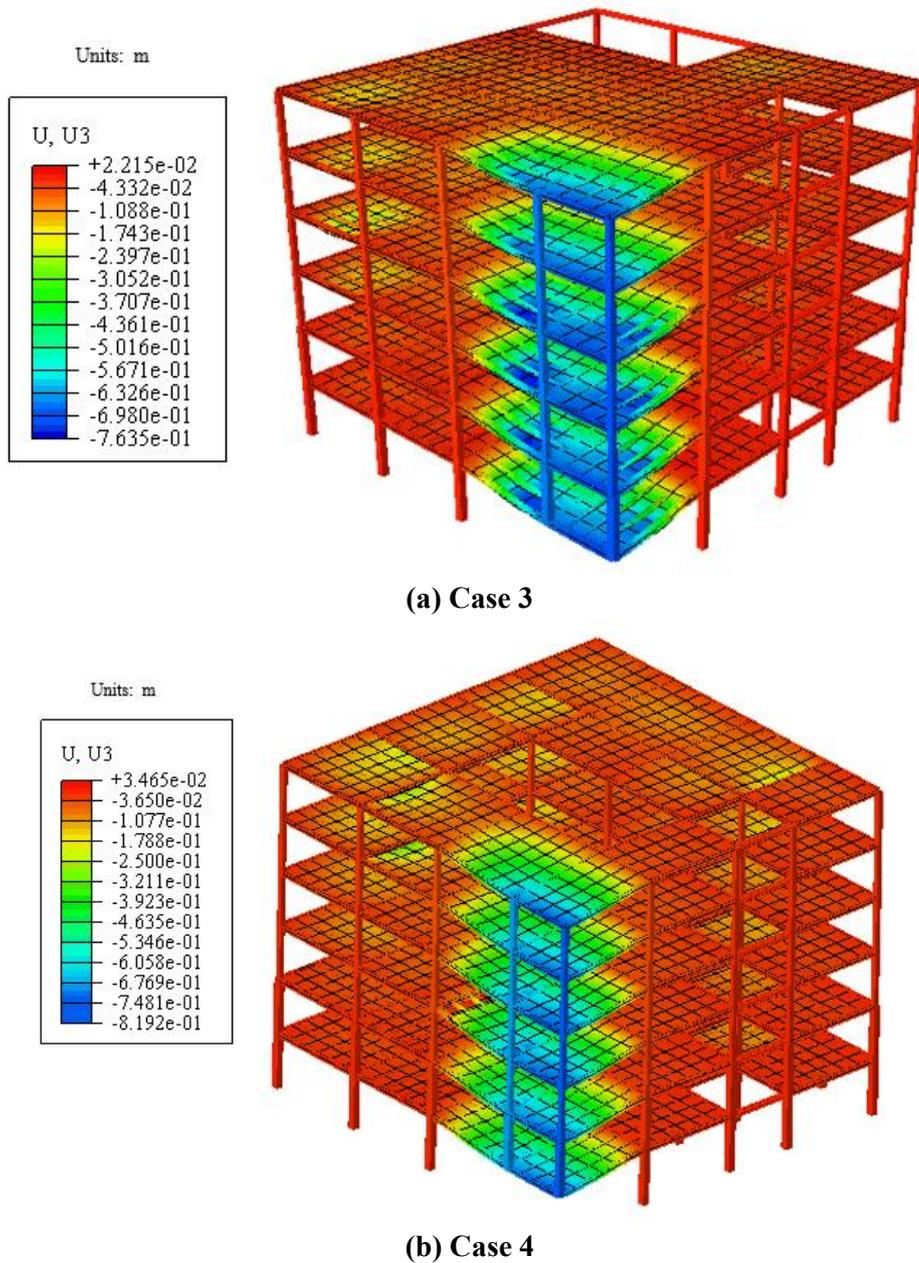
Fig. 16. Displacement contour for cases 3 & 4.
