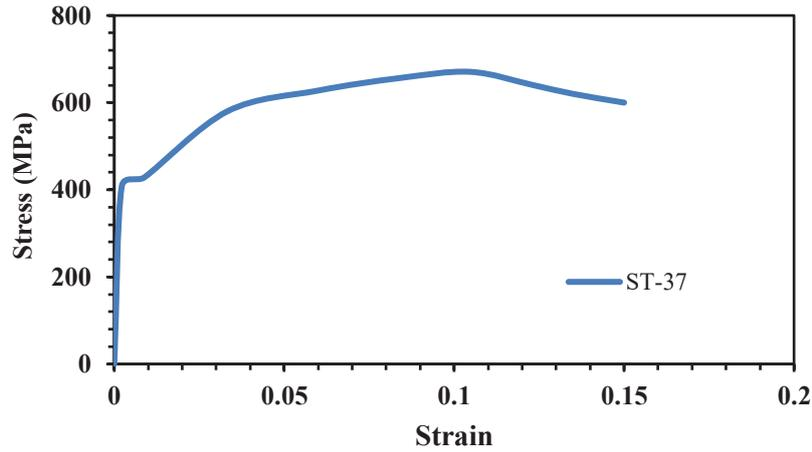
Fig. 2. Stress-strain relationship of steel components.
