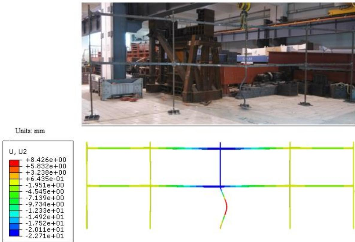
Fig. 11. Final status of the test sample and analysis displacement contour.
