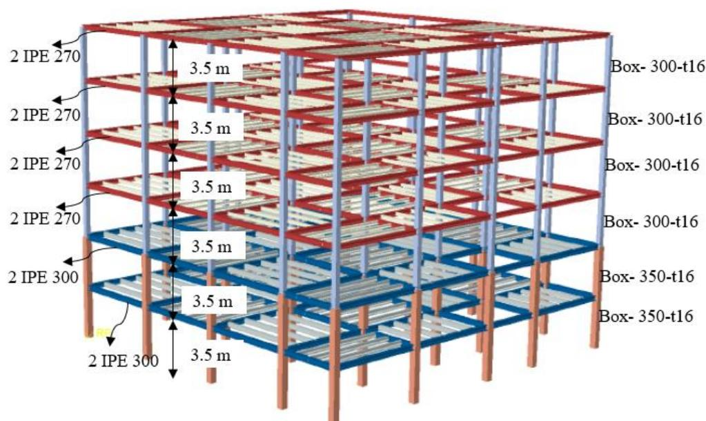
Fig. 4. 3D finite element modeling of a 6-story building.
