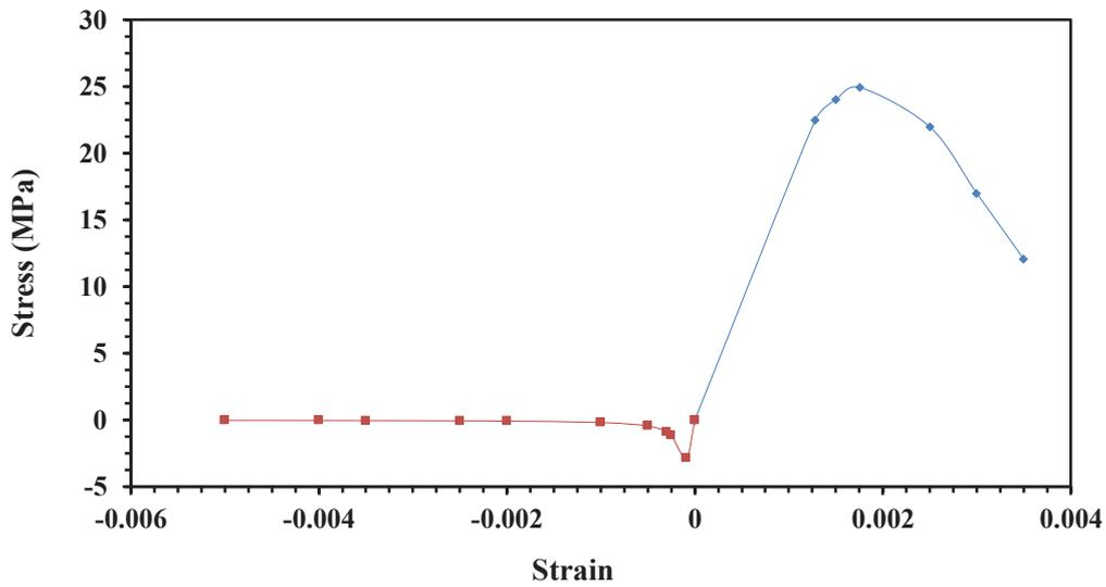
Fig. 3. Stress-strain relationship of concrete components.
