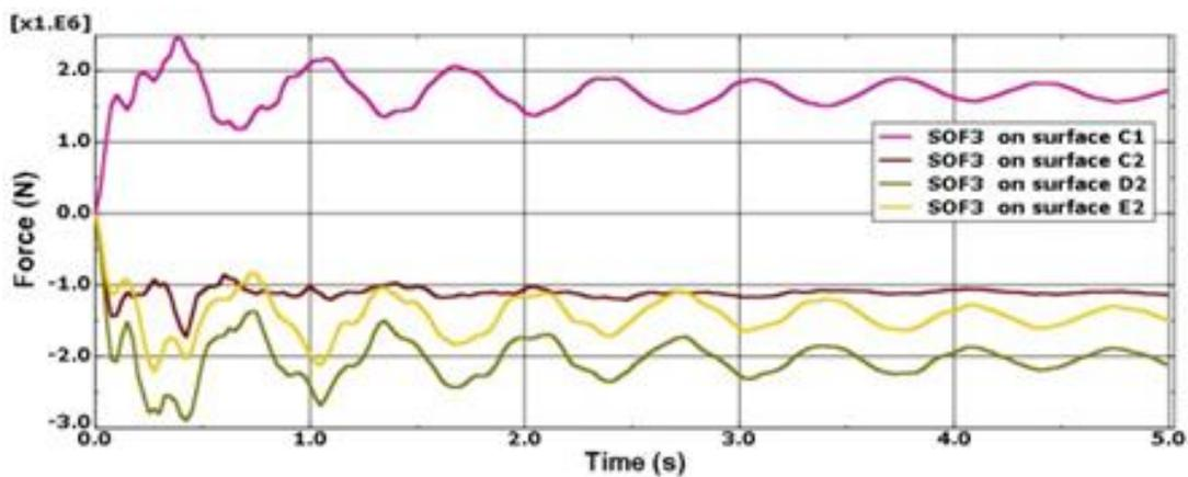
Fig. 15. The exerted load in the members located in the vicinity of the removed column (case 7).
