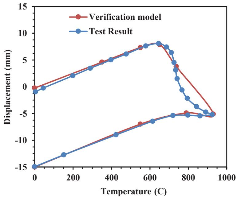
Fig. 12. Displacement result for the point located at the top of the removed column.
