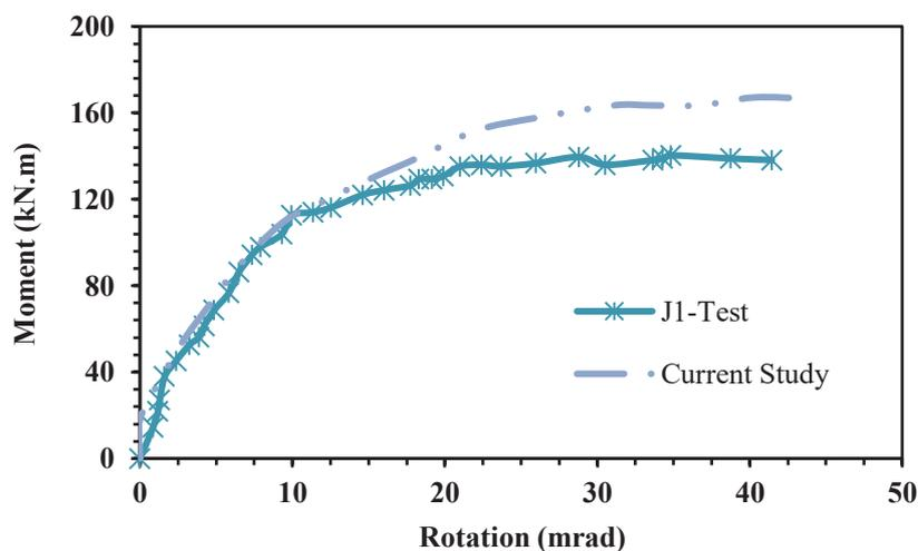
Fig. 9. Moment rotation of finite element and laboratory model [37].
