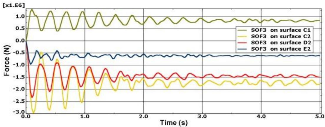
Fig. 13. The exerted load in the members located in the vicinity of the removed column (case 1).
