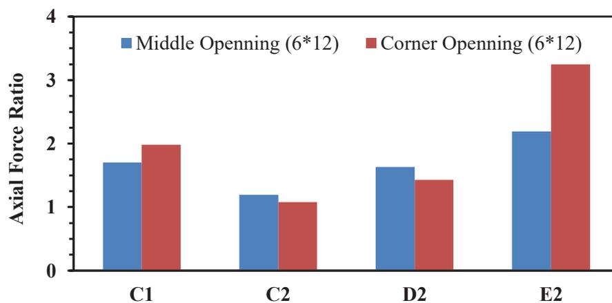
Fig. 17. Effect of the opening location on the openings of dimension (6\*12 m).
