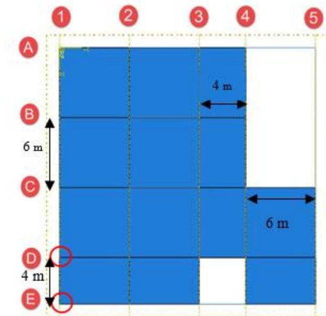
**Fig. 5. The location of the removed columns in the numerical study.**
