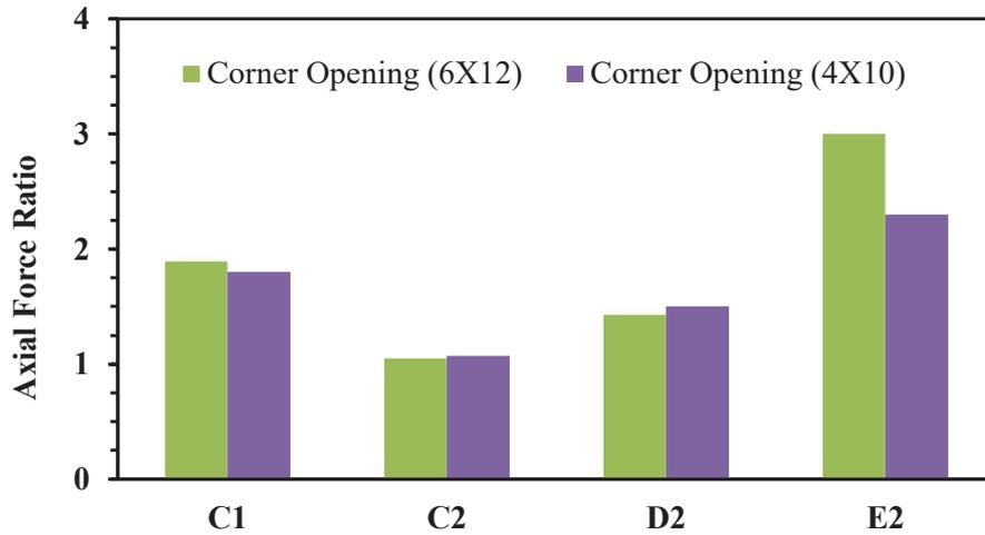
Fig. 19. Effect of the opening dimension on the corner openings.
