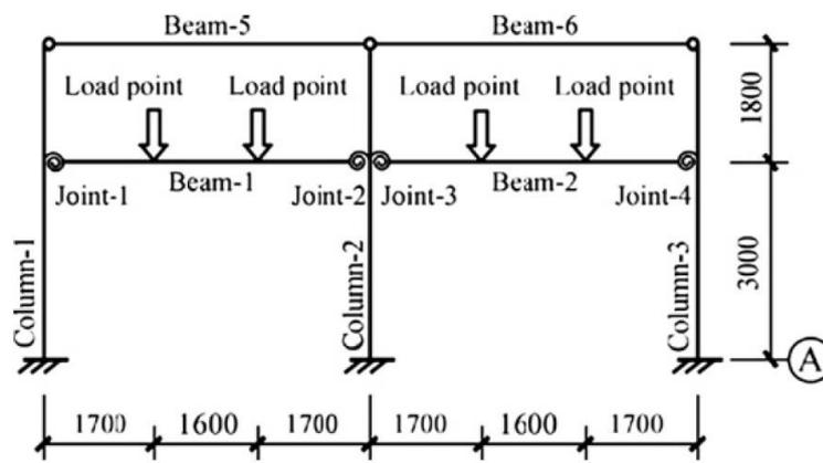
(b) Loading point places at both main frames of the 3D test model, Units in mm.
