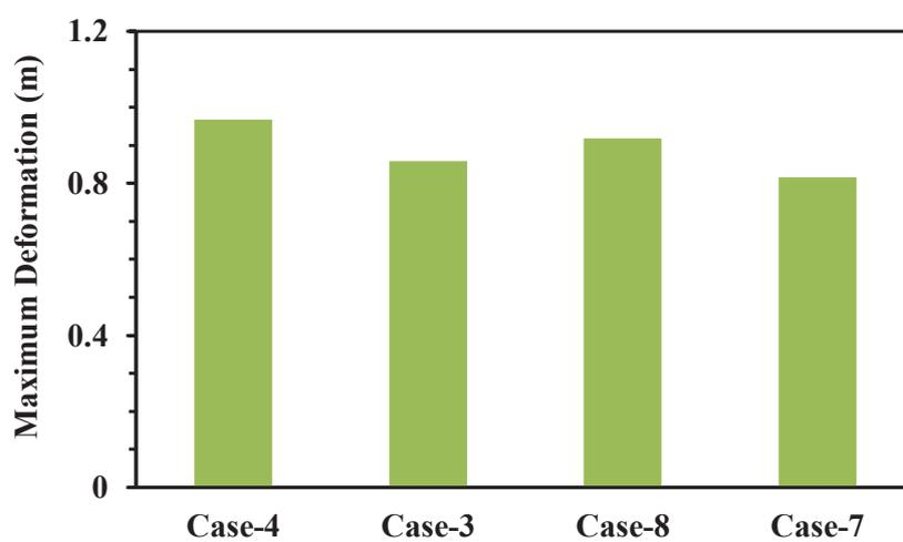
Fig. 22. Effect of the opening dimension and location on the maximum sudden deformation due to column removal.
