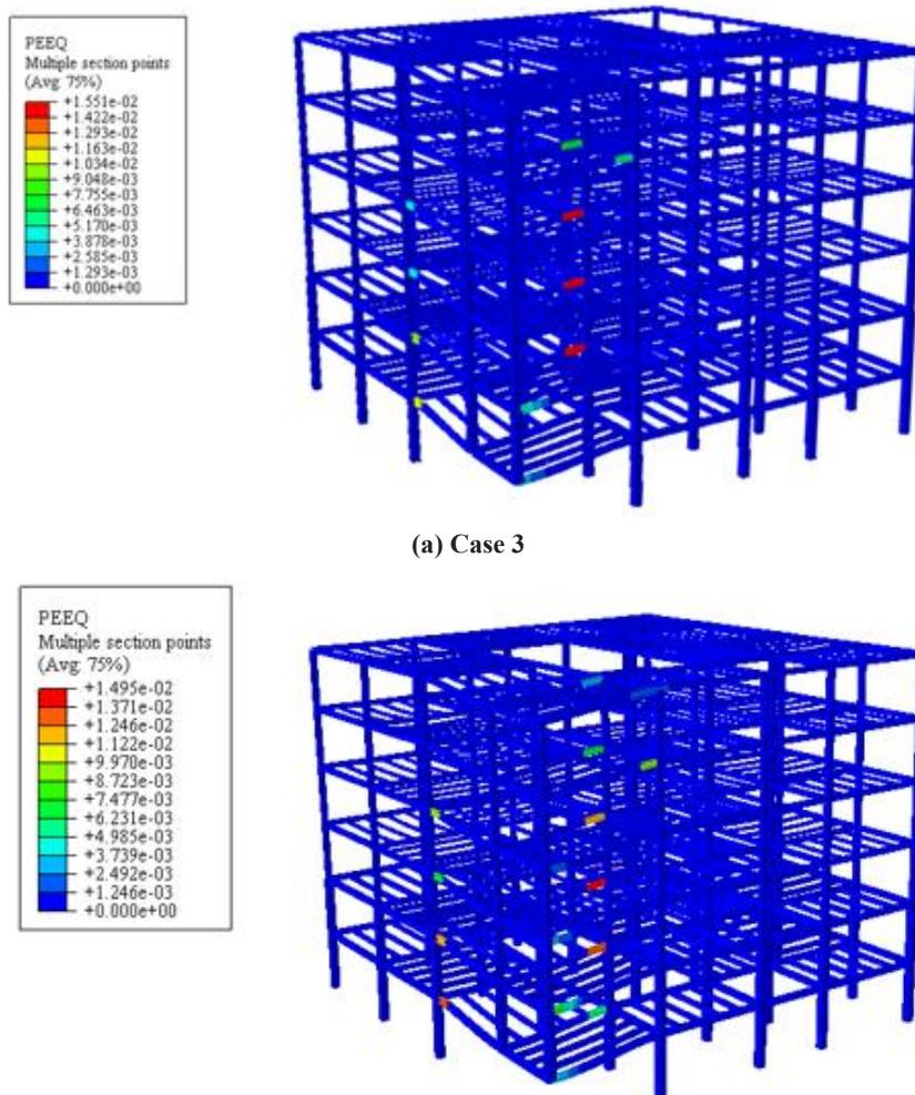
Fig. 21. Plastic Strain contour for cases 3 & 4.
