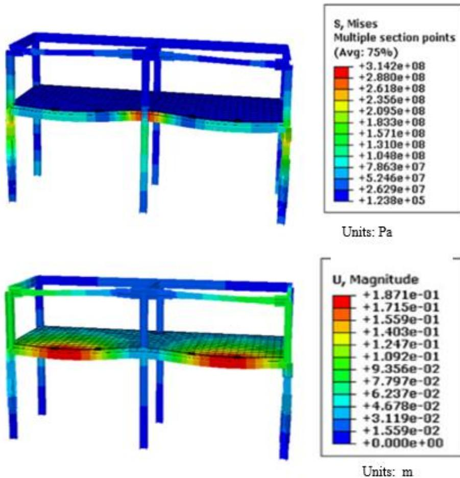
Fig. 8. Stress and displacement results of the verification model in the ABAQUS software.
