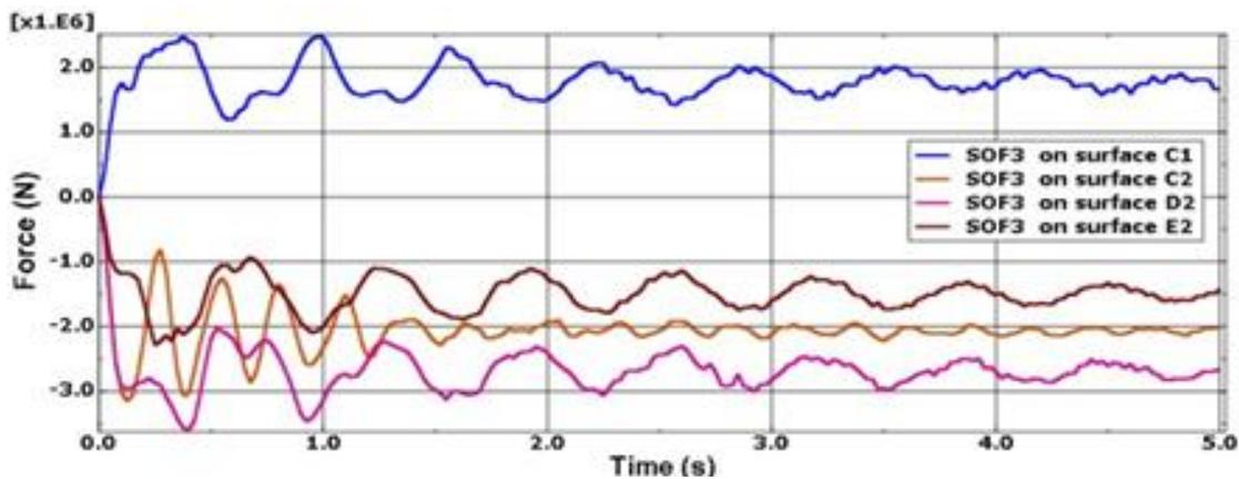
Fig. 14. The exerted load in the members located in the vicinity of the removed column (case 3).
