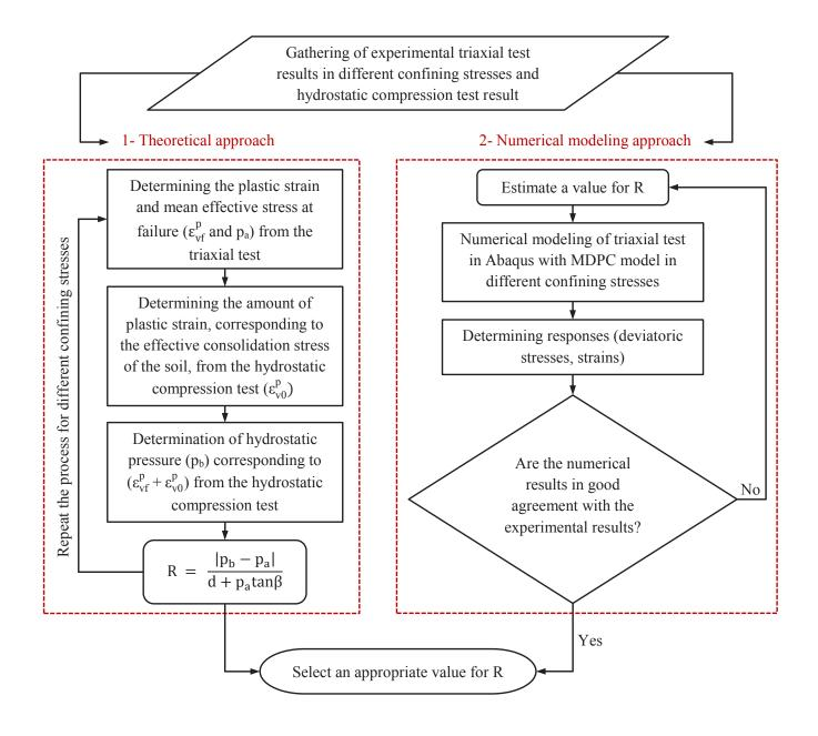
Fig. 7. Procedures for determining the R parameter in the present study.
