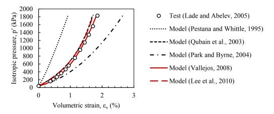
Fig. 5. Measured (prepared by Air Pluviation method) and predicted values for hydrostatic compression of Nevada sand (a) Dr = 30%, and (b) Dr = 70%.
