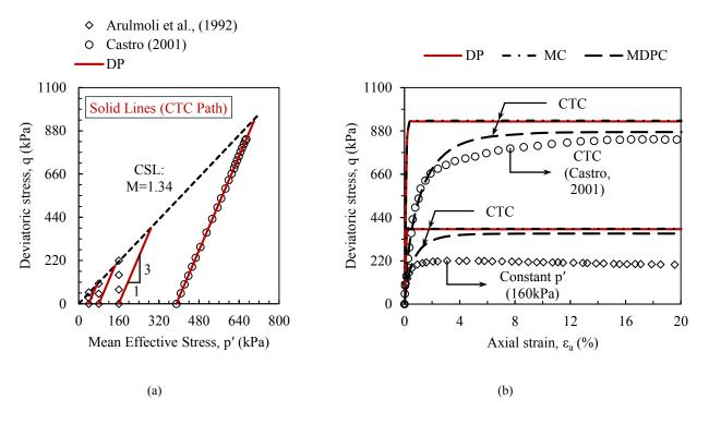
Fig. 13. Comparison of simulation results of conventional triaxial compression test (CTC) with experimental results, (a) stress paths, and (b) (ɛa - q) curves.
