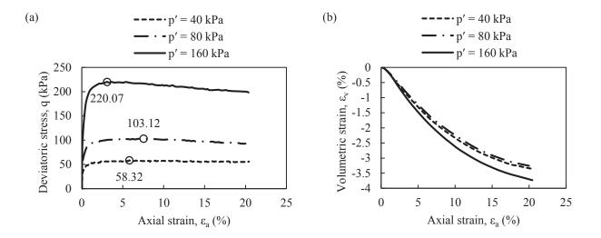
Fig. 9. CD tests results for Nevada sand at a relative density of 40% under effective consolidation stresses of 40, 80, and 160 kPa (a)  $\epsilon a - q$  diagram and (b)  $\epsilon a - \epsilon v$  diagram (Arulmoli et al., 1992).
