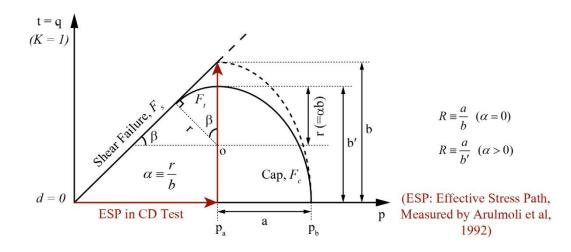
Fig. 8. The stress path in the drained triaxial test of Arulmoli et al. (1992) and the yield surfaces of the MDPC model in the p-t space to determine the R parameter ( $\alpha = 0$ ).
