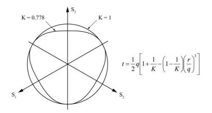
Fig. 3. Modified Drucker-Prager yield surface in the deviatoric principal stress plane (Π-plane).
