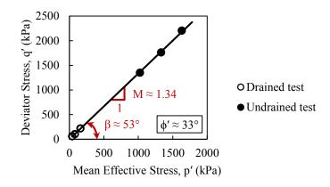
Fig. 2. Drained and undrained triaxial test results for Nevada sand at a relative density of 40% (Arulmoli et al., 1992) [17].
