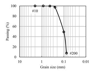
Fig. 1. Grain size distribution curve [17].
