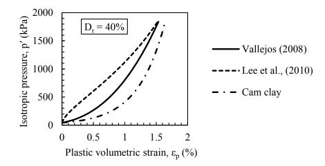
Fig. 6. The volumetric plastic strain of Nevada sand at a relative density of 40%.
