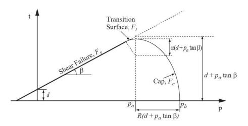
Fig. 4. Yield surface of the MDPC model in the p-t plane [9].
