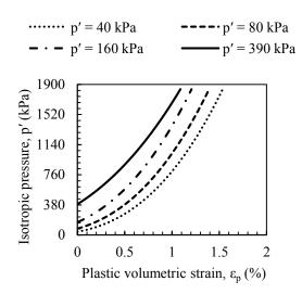
Fig. 11. Hydrostatic compression curves for Nevada sand under different effective consolidation stress based on the Vallejos (2008) model, ( $A_s/p_{atm} = 637$ , b = 1.571,  $a_v = 0.37$ ).
