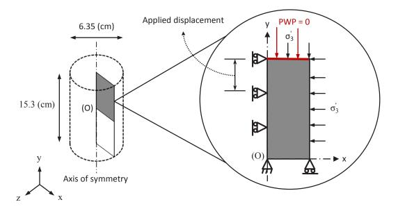
Fig. 10. Axisymmetric finite element model of the drained triaxial test used in Abaqus.
