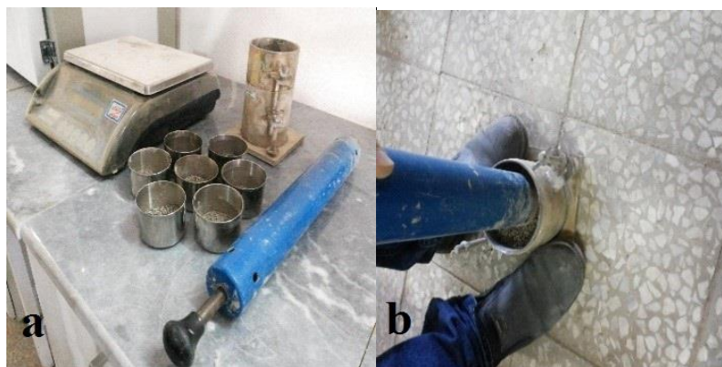
Fig. 4. Compaction test – a: equipment and b: hammering
