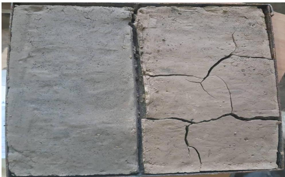
Fig. 11. Results of crack formation over 90 days (Right image: original soil; Left image: soil with 0.07% biochar added).
