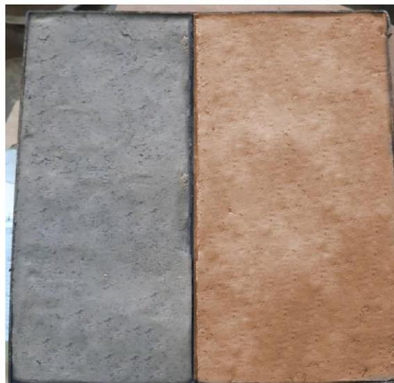
**Fig. 3. Cracking samples on the first day (Right image: original soil; Left image: soil with 0.07% biochar added).**
