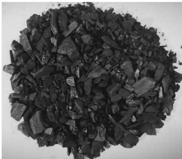
**Fig. 1. Biochar particles after manual crushing and sieving through a No. 40 sieve**
