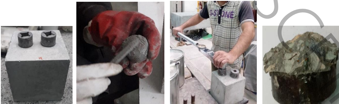
(a) steel cylinder (b) Applying glue on the cylinder (c) the torsional moment (d) the final result
