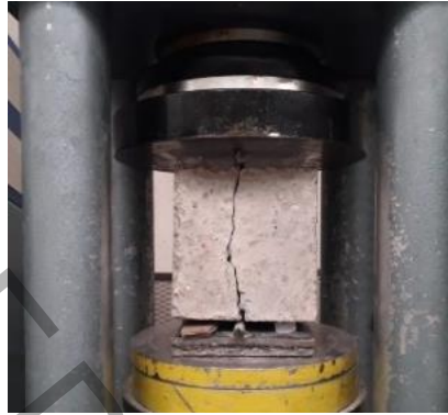
(a) Concrete under the jack
