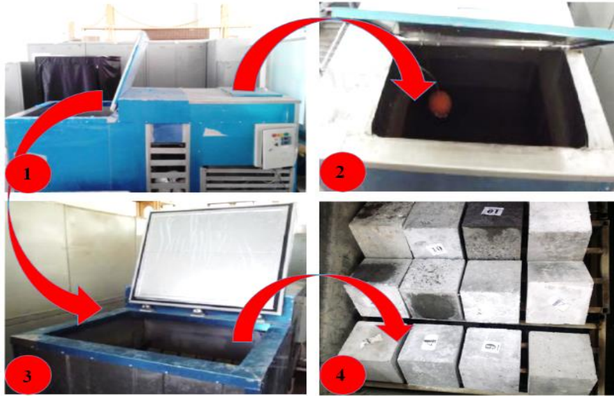
Fig. 17. Placement of cube specimens inside the freeze-thaw machine.
