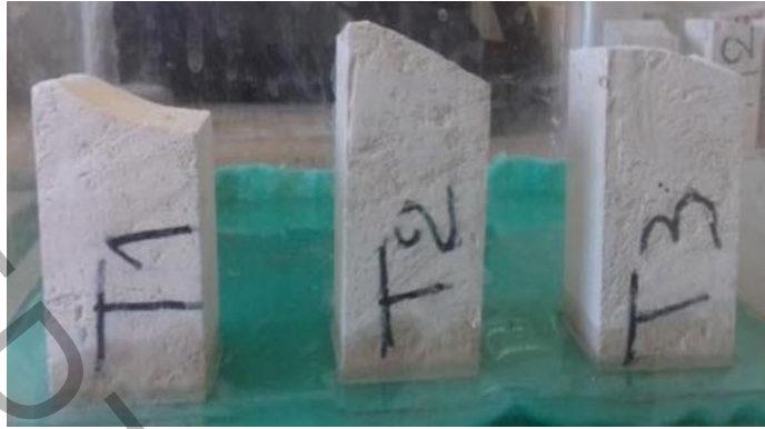
Figure 1. Three Gypsum-Based Composites Incorporating 30% Travertine for Water Absorption capacity analysis
