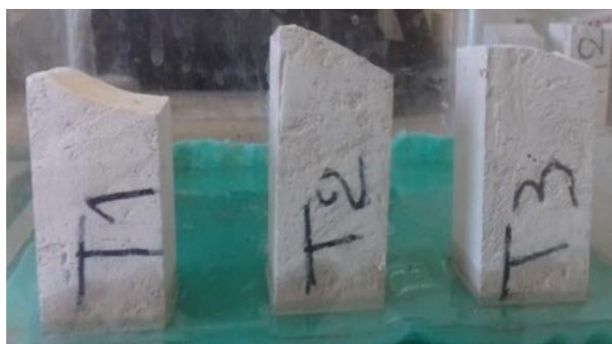
Fig. 1. Three Gypsum-Based Composites Incorporating 30% Travertine for Water Absorption Capacity Analysis
