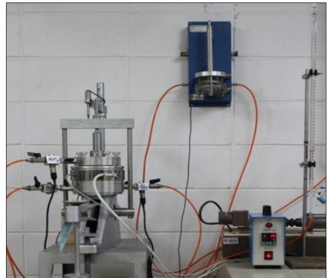
Fig. 5. Assembled system of the modified oedometer
