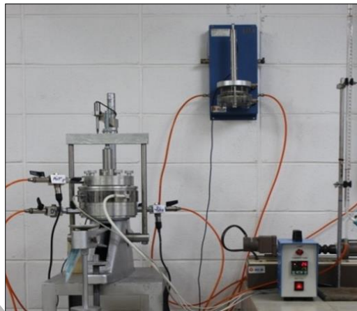
Fig. 5. Assembled system of the modified oedometer
