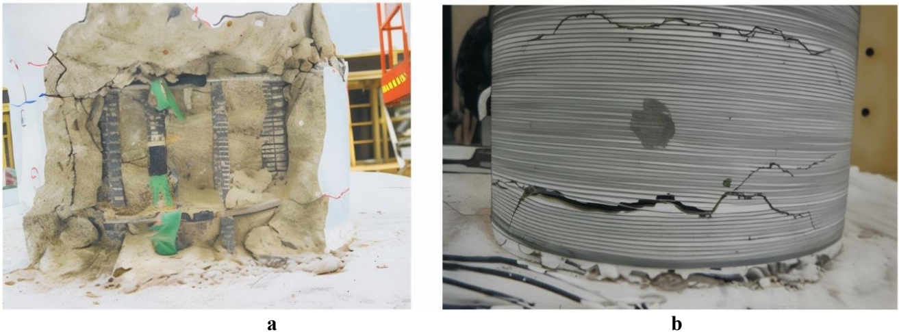
Fig. 16. The column's failure modes with lap splice: a) without SMA wire, b) retrofitting by SMA spiral wires [65].
