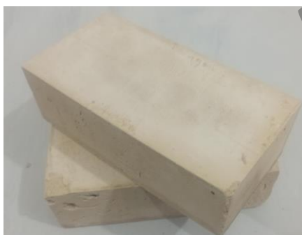
Fig. 4. Unreinforced masonry bricks made of clay, sand, cement and water
