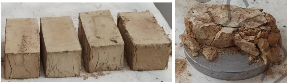
Fig. 11. broken samples under net compression
