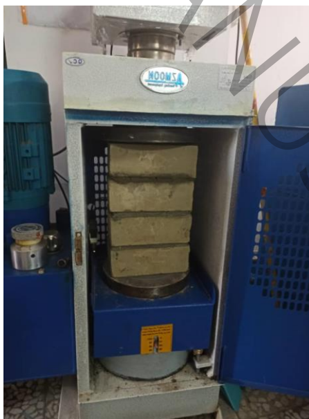
Fig. 13. Masonry prism is constructed using 4 bricks and 3 layers of mortar
