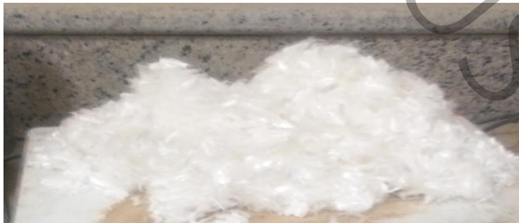
Fig.1: Polypropylene fibers used in the mix.
