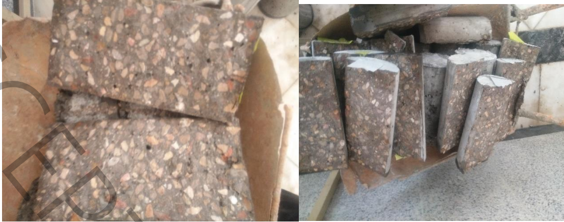
Fig. 15. Concrete sample breaking in the splitting test
