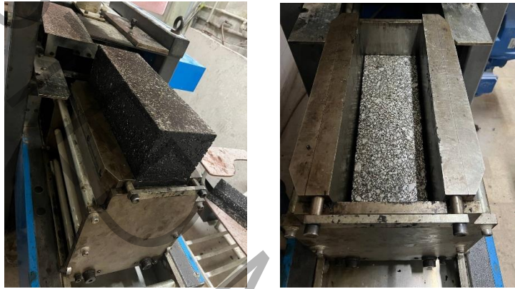
Fig. 3. (a) Compacted sample. (b) Sliced sample
