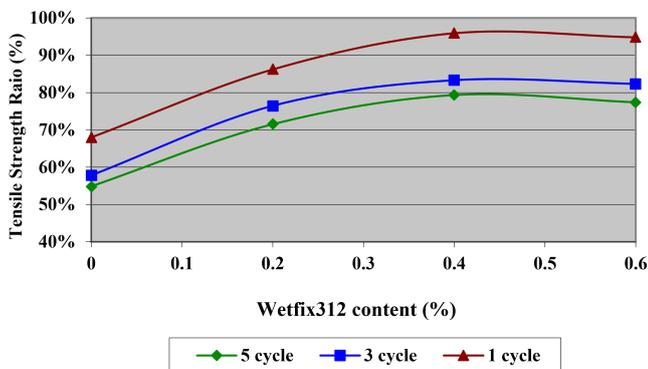
Fig. 9. The effect of freeze–thaw cycles and wexif312 percentage on the TSR (limestone aggregates)
