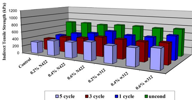
Fig. 3. The relationship between ITS and the type and percentage of additives in different freeze–thaw cycles (limestone aggregate)
