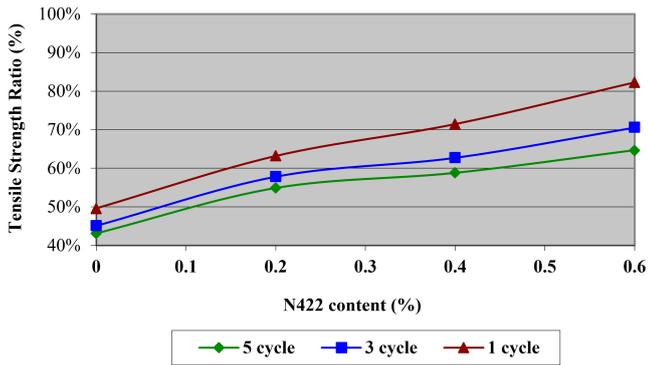
Fig. 7. The effect of freeze–thaw cycles and N422 percentage on the TSR (quartzite aggregates)
