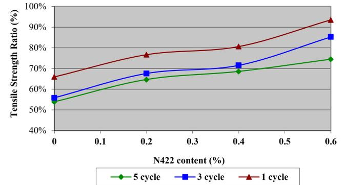
Fig. 5. The effect of freeze–thaw cycles and N422 percentage on the TSR (granite aggregates)
