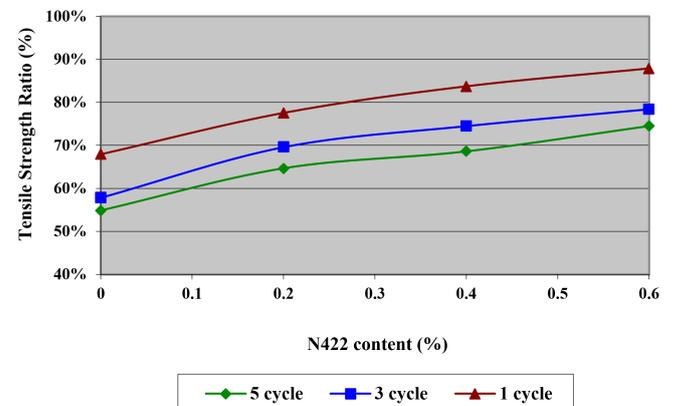
Fig. 6. The effect of freeze–thaw cycles and N422 percentage on the TSR (limestone aggregates)
