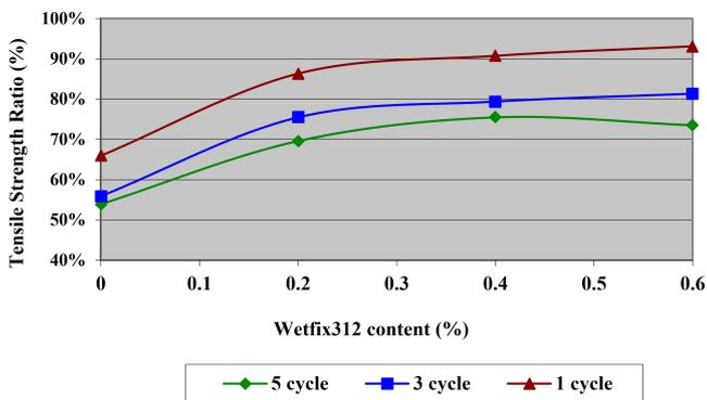
Fig. 8. The effect of freeze–thaw cycles and wexif312 percentage on the TSR (granite aggregates)
