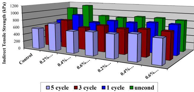
Fig. 2. The relationship between ITS and the type and percentage of additives in different freeze–thaw cycles (granite aggregate)
