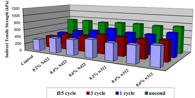
Fig. 4. The relationship between ITS and the type and percentage of additives in different freeze–thaw cycles (quartzite aggregate)
