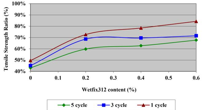
Fig. 10. The effect of freeze–thaw cycles and wexif312 percentage on the TSR (quartzite aggregates)
