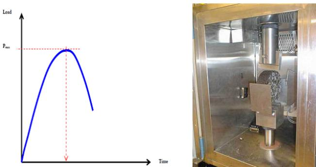
Fig. 1. Test method and loading in ITS test
